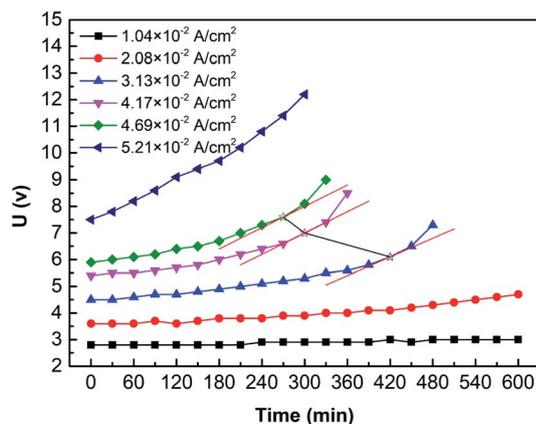
Fig. 11 The curves of the cell voltage over time under various current densities ( $i = 1.04 \times 10^{-2} \text{ A cm}^{-2}$ ,  $2.08 \times 10^{-2} \text{ A cm}^{-2}$ ,  $3.13 \times 10^{-2} \text{ A cm}^{-2}$ ,  $4.17 \times 10^{-2} \text{ A cm}^{-2}$ ,  $4.69 \times 10^{-2} \text{ A cm}^{-2}$ , and  $5.21 \times 10^{-2} \text{ A cm}^{-2}$ ).  $C_{\text{oxime}} = 1.00 \text{ mol L}^{-1}$ .
