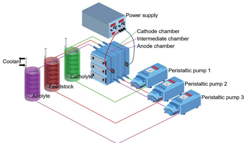
Fig. 3 Experiment equipment of the coupling process.
