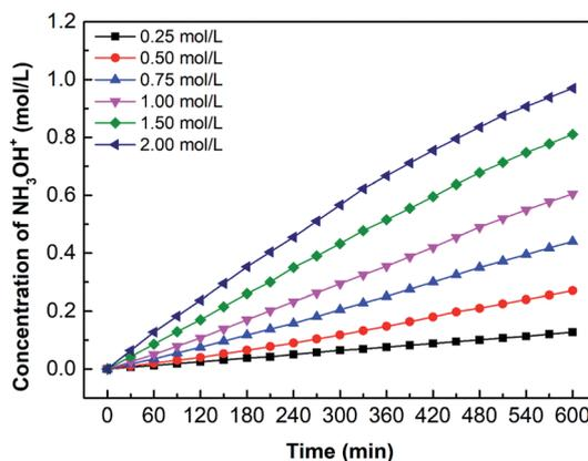
Fig. 12 The curves of hydroxylamine concentration over time for various oxime concentration ( $C_{\text{oxime}} = 0.25 \text{ mol L}^{-1}$ ,  $0.50 \text{ mol L}^{-1}$ ,  $0.75 \text{ mol L}^{-1}$ ,  $1.00 \text{ mol L}^{-1}$ ,  $1.50 \text{ mol L}^{-1}$ , and  $2.00 \text{ mol L}^{-1}$ ).  $i = 4.69 \times 10^{-2} \text{ A cm}^{-2}$ .
