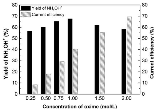
Fig. 10 The effect of oxime concentration on the yield of hydroxylamine and current efficiency.  $i = 4.69 \times 10^{-2} \text{ A cm}^{-2}$ , time = 600 min, and concentration of  $\text{H}_2\text{SO}_4$  equals  $1.00 \text{ mol L}^{-1}$ .
