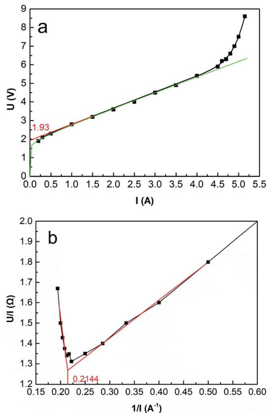
Fig. 5 (a) Initial cell voltage versus current intensity.  $C_{\text{oxime}} = 1.00$  mol L<sup>-1</sup>, mass velocity = 135.0 g min<sup>-1</sup>,  $T = 25$  °C. (b)  $R - 1/I$  curve.
