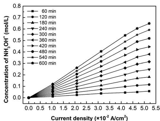
Fig. 7 The effect of current density on the hydroxylamine concentration.  $C_{\text{oxime}} = 1.00 \text{ mol L}^{-1}$ .
