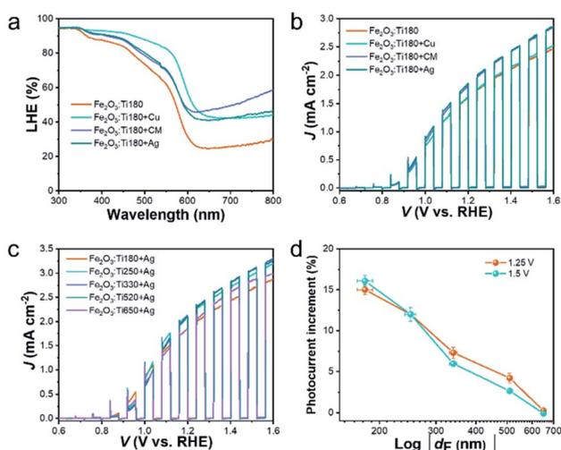
**Fig. 4** (a) LHE and (b) polarization curve of the bare Fe<sub>2</sub>O<sub>3</sub>:Ti<sub>180</sub> electrode and those supported by Cu foil, Ag foil and commercial mirror (CM); (c) the polarization curves of the Fe<sub>2</sub>O<sub>3</sub>:Ti electrodes with Ag back-reflector; (d) the calculated photocurrent density increment at certain bias potentials as a function of the logarithm of film thickness ( $d_p$ ) thanks to the light reflection of Ag foil.
