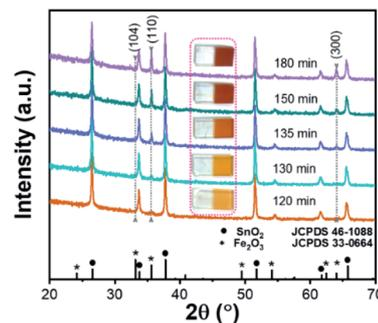
Fig. 1 XRD patterns and photographs (inset) of the Fe<sub>2</sub>O<sub>3</sub>:Ti electrodes prepared by adjusting the hydrothermal time.
