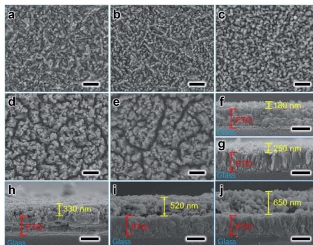
Fig. 2 Verticle (a–e) and cross-section (f–j) SEM view of the Fe<sub>2</sub>O<sub>3</sub>:Ti electrodes prepared by adjusting the hydrothermal time; (a and f) 120 min; (b and g) 130 min; (c and h) 135 min; (d and i) 150 min; (e and j) 180 min. Scale bars are 500 nm.
