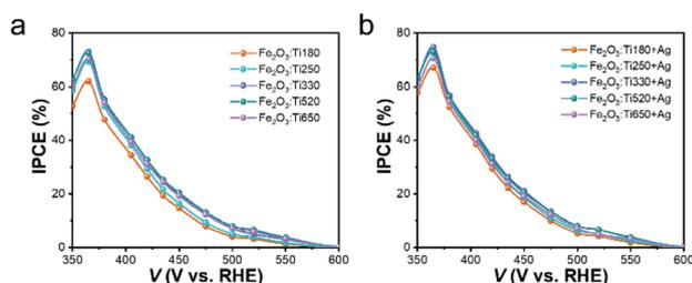
Fig. 5 Comparison of the incident photon-to-electron conversion efficiency (IPCE) of the  $\text{Fe}_2\text{O}_3:\text{Ti}$  electrodes of different thicknesses (a) with and (b) without Ag back-reflector.
