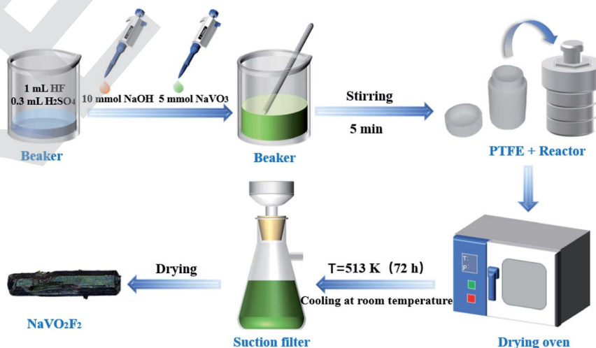
Fig. 1 Schematic of the process for preparing \text{NaVO}_2\text{F}_2 .
