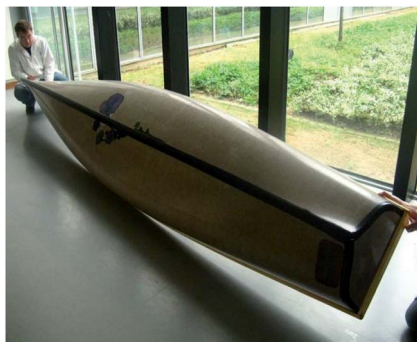
Fig. 2 Flax/PLA canoe manufactured during the NAVECOMAT project.
