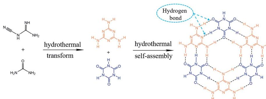
Fig. 4 Schematic illustration for the fabrication of MCA during hydrothermal process.
