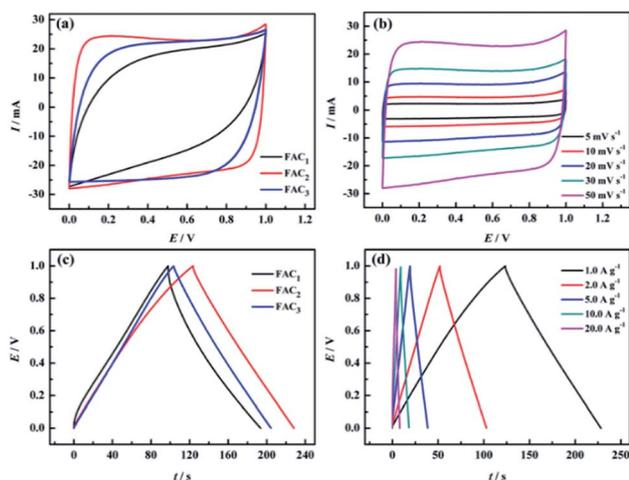
Fig. 6 Electrochemical performance of FAC<sub>X</sub> measured in two-electrode system in 6.0 M KOH electrolyte. (a) CV curves of FAC<sub>1</sub>, FAC<sub>2</sub> and FAC<sub>3</sub> at 50 mV s<sup>-1</sup>; (b) CV curves of FAC<sub>2</sub> at different scan rates; (c) GCD curves of FAC<sub>1</sub>, FAC<sub>2</sub> and FAC<sub>3</sub> at 1.0 A g<sup>-1</sup>; (d) GCD curves of FAC<sub>2</sub> at different current densities.
