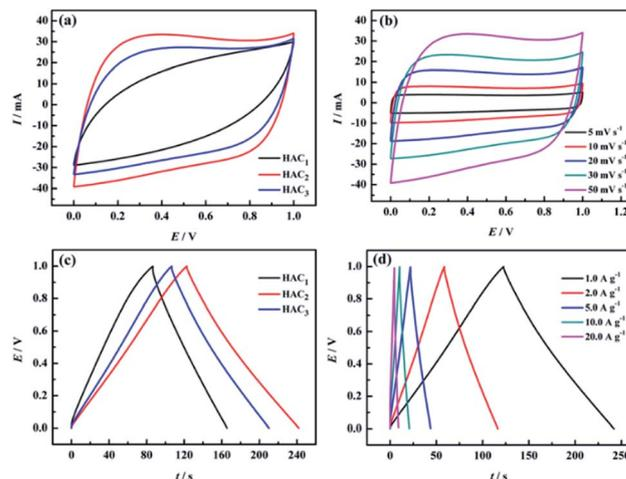
Fig. 7 Electrochemical performance of HAC<sub>X</sub> measured in two-electrode system in 6.0 M KOH electrolyte. (a) CV curves of HAC<sub>1</sub>, HAC<sub>2</sub> and HAC<sub>3</sub> at 50 mV s<sup>-1</sup>; (b) CV curves of HAC<sub>2</sub> at different scan rates; (c) GCD curves of HAC<sub>1</sub>, HAC<sub>2</sub> and HAC<sub>3</sub> at 1.0 A g<sup>-1</sup>; (d) GCD curves of HAC<sub>2</sub> at different current densities.
