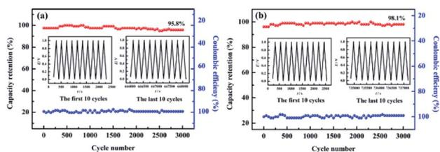
Fig. 10 Cycling stability and coulombic efficiency of (a)  $\text{FAC}_2$  and (b)  $\text{HAC}_2$  electrodes at  $1.0 \text{ A g}^{-1}$  for 3000 cycles. Inset: the GCD curves of the first and last ten cycles.
