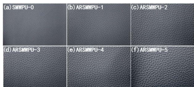
Fig. 10 Effect of different polysiloxane contents modifying self-matting WPU on gloss of the leather coating.
