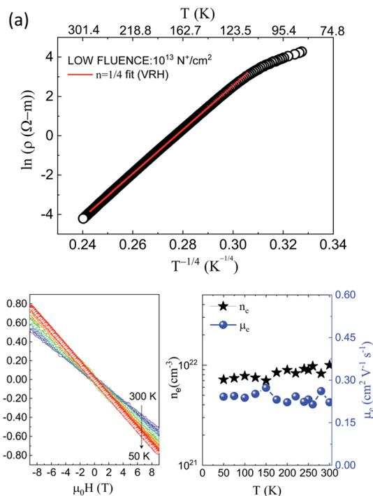
**Fig. 7** (a)  $\ln \rho$  vs.  $T^{-0.25}$  plot for UNCD implanted at low fluence showing insulating behaviour and exhibiting VRH mechanism of transport, (b) Hall resistivity vs. applied field (left) showing n-type conduction and the corresponding electron concentration and its respective mobility at various temperatures (right) for UNCD implanted at medium fluence which is semiconducting in nature.
