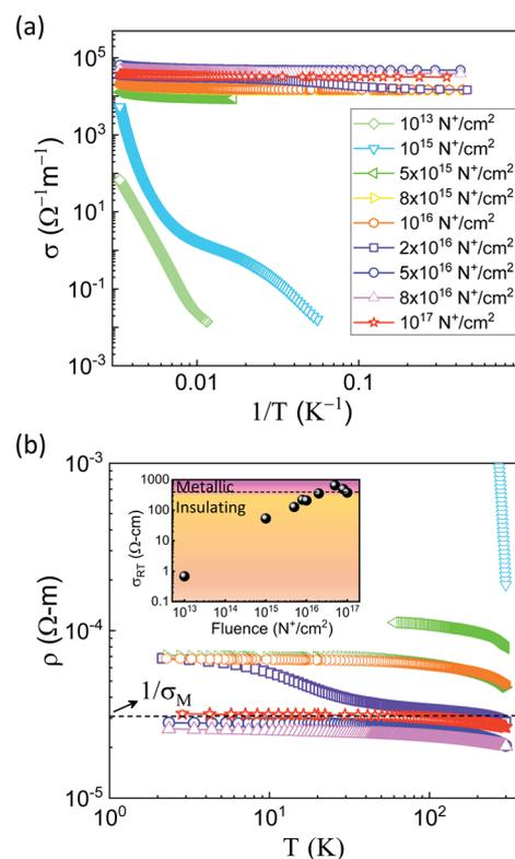
Fig. 6 Plot of (a) conductivity *versus* inverse temperature for UNCDs implanted with various fluences and (b) temperature variation of resistivity depicting that transition from insulating to semi-metallic behaviour of transport property.
