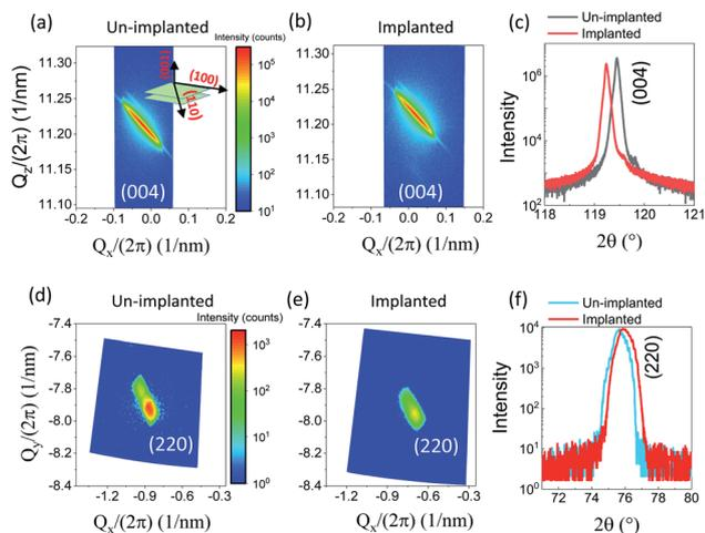
Fig. 4 RSM in (a) and (b) out-of-plane mode for the (004) symmetric reflection and (d) and (e) in-plane mode for (220) asymmetric reflection for un-implanted and implanted SCDs respectively and (c) and (f) show the  $2\theta$  scan of the (004) and (220) reflection in out-of-plane and in-plane configuration respectively.
