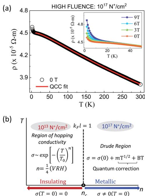
Fig. 8 (a) Resistivity versus temperature plot for UNCD implanted with high fluence *i.e.*  $10^{17} \text{ cm}^{-2}$  (semi-metallic) where the QCC (quantum corrections for conductivity model) fits properly from 300 K to 10 K and below 10 K and (b) a schematic illustration of the conduction mechanism in UNCDs with various ion fluences.
