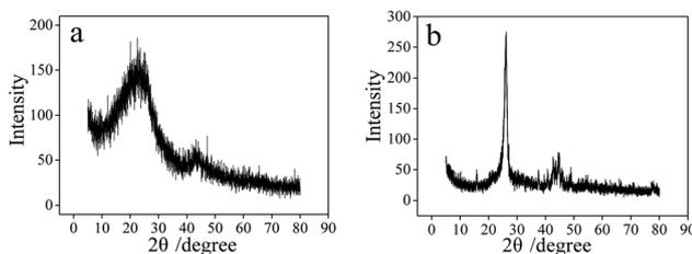
Fig. 8 XRD diffraction patterns of the carbon materials: (a) CSs prepared in Li–Na eutectic with 1 wt% SnO<sub>2</sub>, (b) CNTs prepared in 750 °C Li<sub>2</sub>CO<sub>3</sub> electrolyte.
