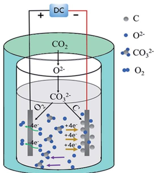
Scheme 1 Schematic diagram of the experimental process.
