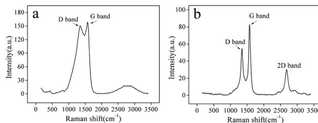
Fig. 9 Raman spectrum of the carbon materials: (a) CSs prepared in Li–Na eutectic with 1 wt% SnO<sub>2</sub>, (b) CNTs prepared in Li<sub>2</sub>CO<sub>3</sub> electrolyte.
