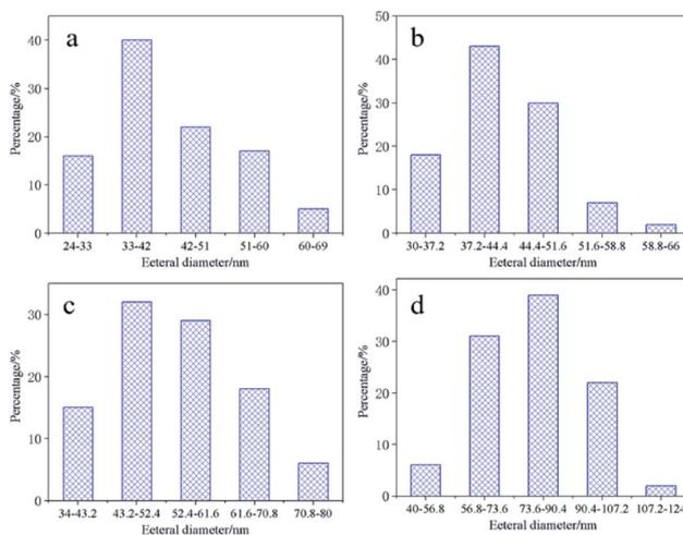
**Fig. 5** The outer diameter distribution of CNTs obtained under different current densities in 750 °C  $Li_2CO_3$  electrolyte (a)  $50\text{ mA cm}^{-2}$ , (b)  $100\text{ mA cm}^{-2}$ , (c)  $200\text{ mA cm}^{-2}$ , (d)  $300\text{ mA cm}^{-2}$ .
