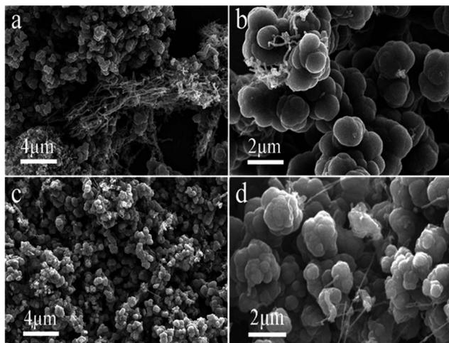
Fig. 6 SEM images of the carbon products generated in 750 °C Li–Na (1 : 1 wt) eutectic: (a and b) 1 wt% SnO<sub>2</sub>, (c and d) 1 wt% GeO<sub>2</sub>.
