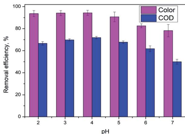
Fig. 2 Effect of pH value on color and COD removal efficiency of DWTS at  $J = 10.0 \text{ mA cm}^{-2}$ ,  $t = 60 \text{ min}$ ,  $d = 4.0 \text{ cm}$ ;  $m_{\text{DWTS}} = 1.0 \text{ g}$  and  $T = 25^\circ \text{C}$ . The error bars represent standard deviation.
