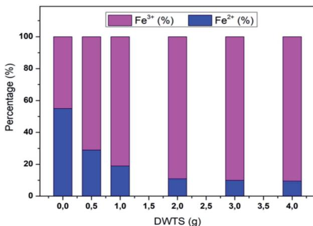
Fig. 7 Percentage distribution of  $\text{Fe}^{2+}/\text{Fe}^{3+}$  ions before and after EFP reactions by using DWTS.
