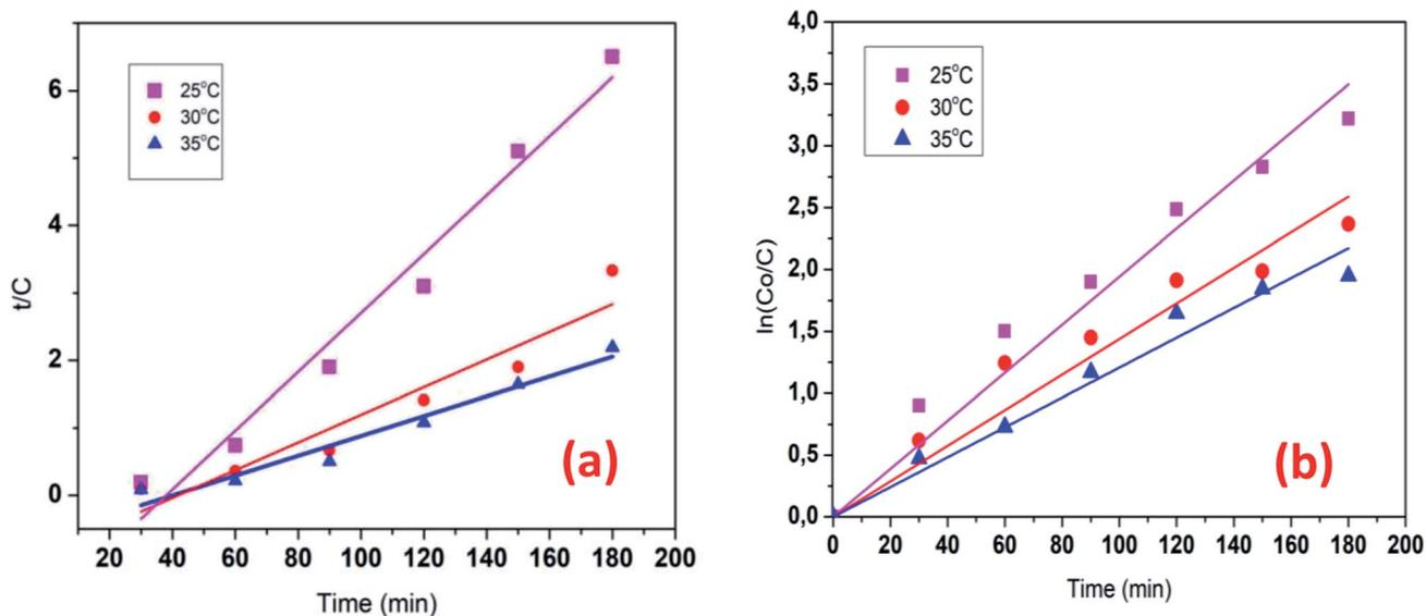
Fig. 9 Reaction kinetics plot for differential temperature: pseudo first-order (a) pseudo-second-order (b) model for the COD degradation. Conditions:  $V = 500$  mL,  $J = 14.0$  mA  $\text{cm}^{-2}$ ,  $t = 90$  min,  $m_{\text{DWTs}} = 2.0$  g, and  $\text{pH} = 4.0$ . The symbol are the experimental data. The curve (a) presents the corresponding kinetics analysis assuming a pseudo first-order reaction, the curve (b) presents pseudo second-order reaction.
