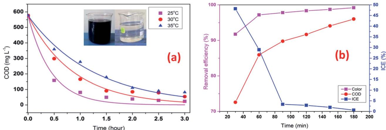
Fig. 8 Effect of temperature (a) on COD degradation; operating time (b) on decolorization and COD degradation efficiency at  $J = 14 \text{ mA cm}^{-2}$ ,  $t = 60 \text{ min}$ ,  $m_{\text{DWTs}} = 2.0 \text{ g}$ , and  $\text{pH} = 4.0$ . Symbols are experimental data. The curve (a) presents the corresponding kinetics analysis assuming a pseudo first-order reaction.
