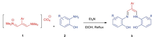
Scheme 2 Synthesis of Schiff bases 3 via the reaction between trimethinium salts 1 and diverse aminophenols 2 in the presence of \text{Et}_3\text{N} in EtOH at reflux.
