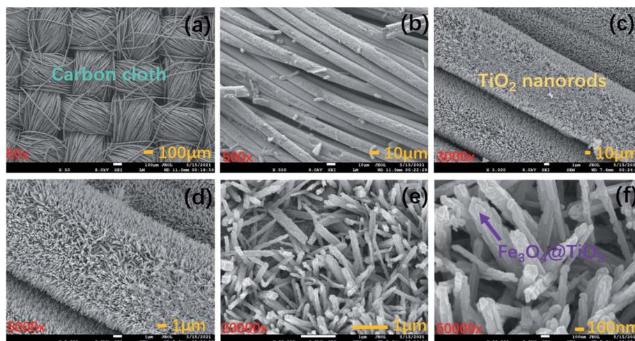
Fig. 2 (a)–(d) Low magnification SEM images of  $\text{Fe}_3\text{O}_4/\text{TiO}_2@\text{C}-3$ , and (e) and (f) high magnification SEM images of  $\text{Fe}_3\text{O}_4/\text{TiO}_2@\text{C}-3$  composite.
