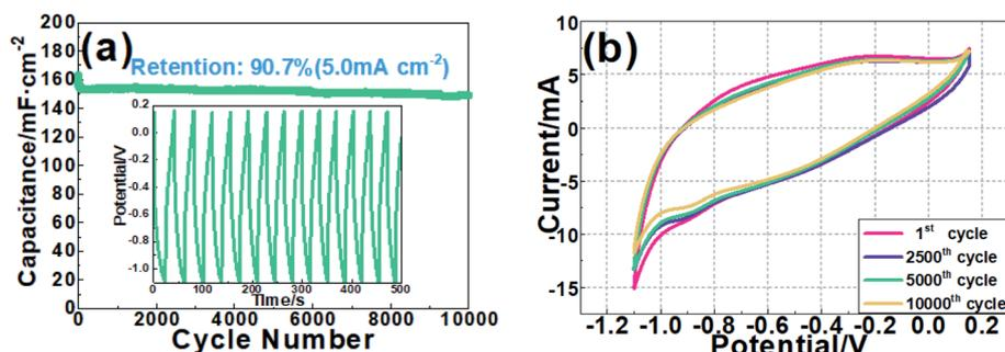
Fig. 6 (a) Cycling stability of the Fe<sub>3</sub>O<sub>4</sub>/TiO<sub>2</sub>@C-3 electrode, (b) comparable CV measurement at various cycle stages.
