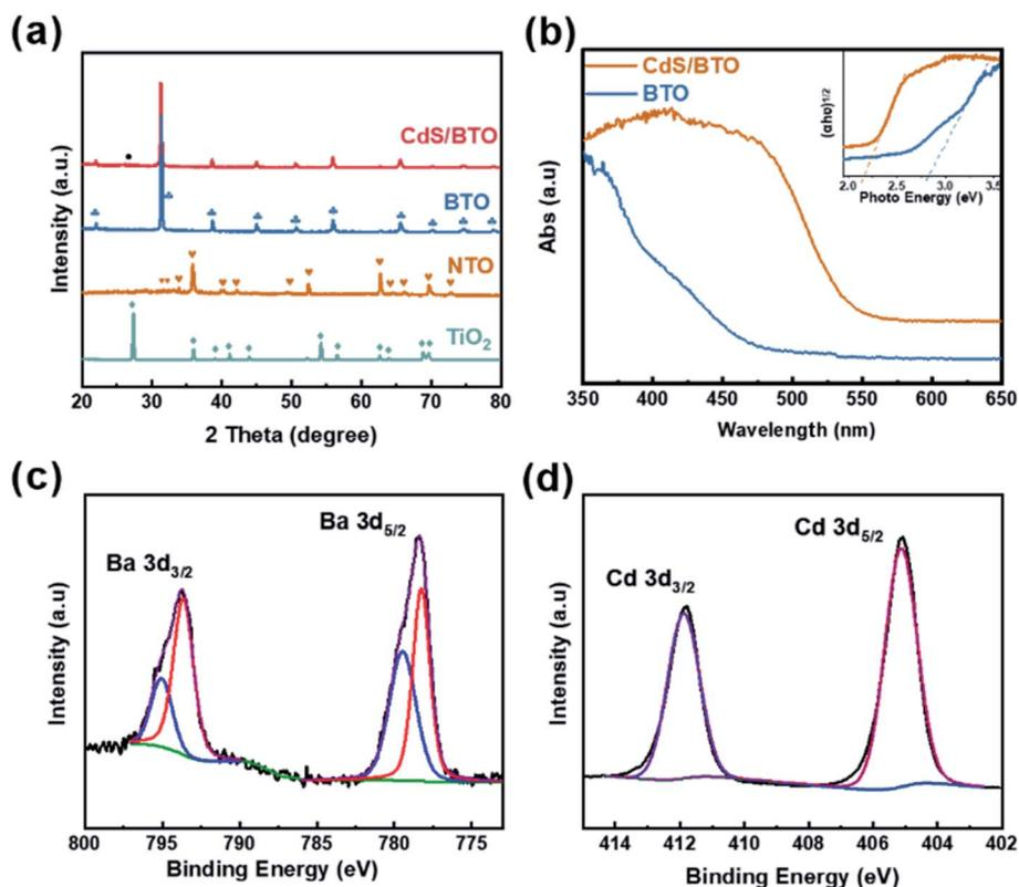
Fig. 2 (a) XRD patterns of the TiO<sub>2</sub>, NTO, BTO and CdS/BTO NWs samples. (b) UV-vis absorption spectra and the inset in (b) presents the corresponding plots of  $(\alpha h\nu)^2$  vs. photon energy. XPS spectra of the CdS/BTO NWs samples: (c) Ba 3d and (d) Cd 3d peaks.
