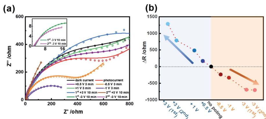
Fig. 5 (a) EIS Nyquist plots of the CdS/BTO NWs samples after different polarizations and the inset shows the results for  $-3$  V (1 $^{\text{st}}$ ) and  $-3$  V (2 $^{\text{nd}}$ ). Open circles were test data points and solid lines were corresponding fitting. (b) Impedance change value compared to unpolarized sample of the CdS/BTO NWs samples.
