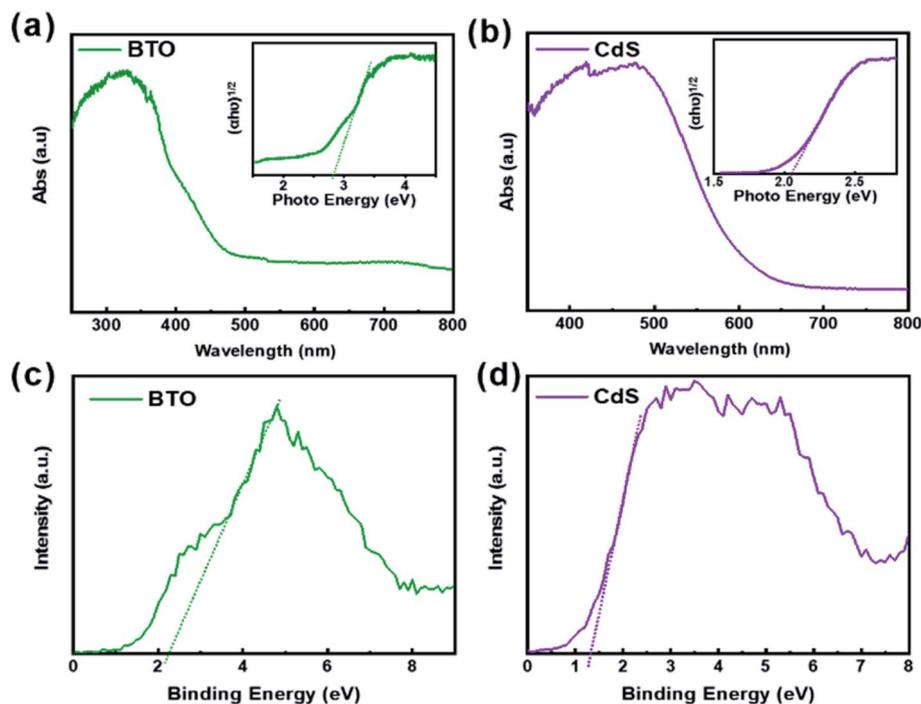
Fig. 8 UV-vis absorption spectra of (a) BTO and (b) CdS. The insets in (a and b) present the corresponding plots of  $(\alpha h\nu)^{1/2}$  vs. photon energy. Valence-band XPS spectra of (c) the BTO and (d) CdS samples.
