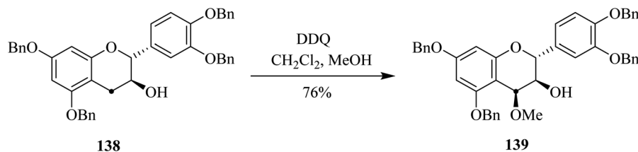
Scheme 49 Conversion of catechin to flavanol analog by DDQ.
