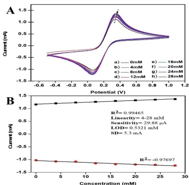
Fig. 8 (A) Electrochemical sensing of AA with varying the concentration (4–28 mM) by the bT-ZnO/ITO electrode in 50 mM PBS (pH 7, 0.9% NaCl) containing 5 mM  $[\text{Fe}(\text{CN})_6]^{3-/4-}$  at scan rate of  $50 \text{ mV s}^{-1}$ . (B) Calibration curve of the bT-ZnO/ITO electrode with varying the current as a function of the AA concentration (4–28 mM) in 50 mM PBS (pH 7, 0.9% NaCl) containing 5 mM  $[\text{Fe}(\text{CN})_6]^{3-/4-}$  at a scan rate of  $50 \text{ mV s}^{-1}$ .
