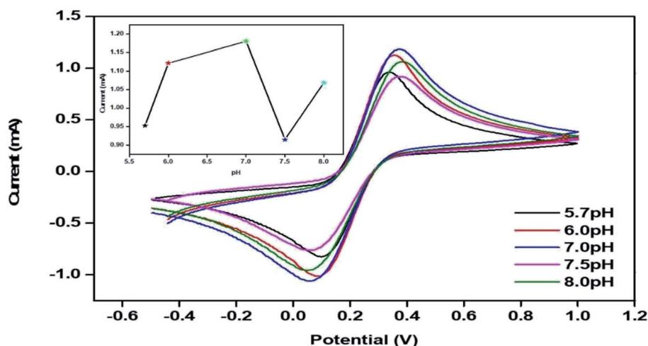
Fig. 7 CV of the bT-ZnO/ITO electrode with varying the pH (5.7 to 8) of 50 mM PBS (0.9% NaCl) containing 5 mM  $[\text{Fe}(\text{CN})_6]^{3-/4-}$ ; the inset shows the current response of the bT-ZnO/ITO electrode as a function of the pH.
