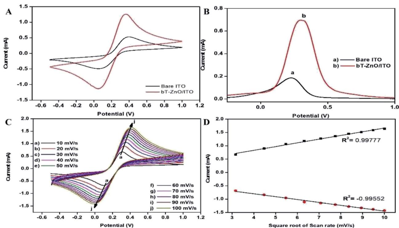
Fig. 6 (A) CV and (B) DPV of the bare ITO (black curve), and bT-ZnO/ITO (red curve), (C) CV curve of bT-ZnO/ITO at varying scan rates (10–100  $\text{mV s}^{-1}$ , pH 7) at 27 °C. (D) Increasing current vs. difference in the potential as a function of the square root of the scan rate (10–100  $\text{mV s}^{-1}$ ).
