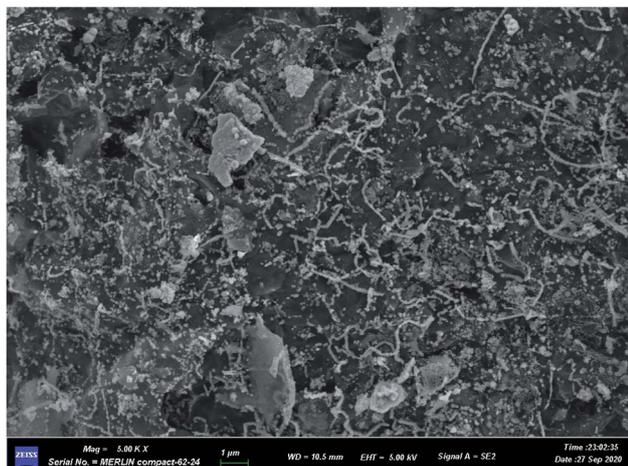
Fig. 1 An SEM image of the Fe<sup>0</sup>/GO composite.
