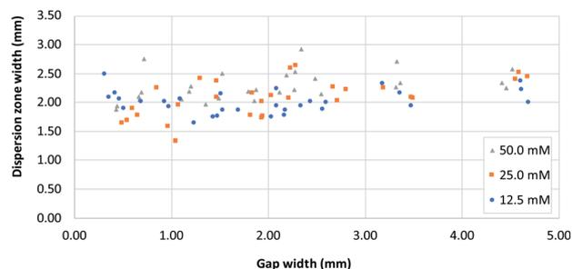
Fig. 5 A plot of dispersion zone width before the gap (*i.e.* at dispersion profile line, Fig. 1B) in systems with different gap widths, for three different reagent concentrations.  $[\text{Fe}^{2+}]$  and  $[\text{SCN}^-]$  were equal in all experiments.
