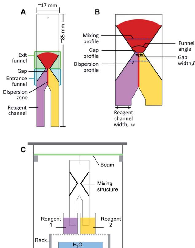
**Fig. 1** Schematic representations of (A) the paper structure proposed for the passive mixing of liquids on paper, (B) an expanded view of the hourglass structure, showing the design parameters and (C) the experimental setup. Experiments are conducted with the paper devices positioned vertically. Flow of solutions in all schematics is from the bottom to the top, where pink and yellow colours represent reagent solutions, and red the solution of reaction product.
