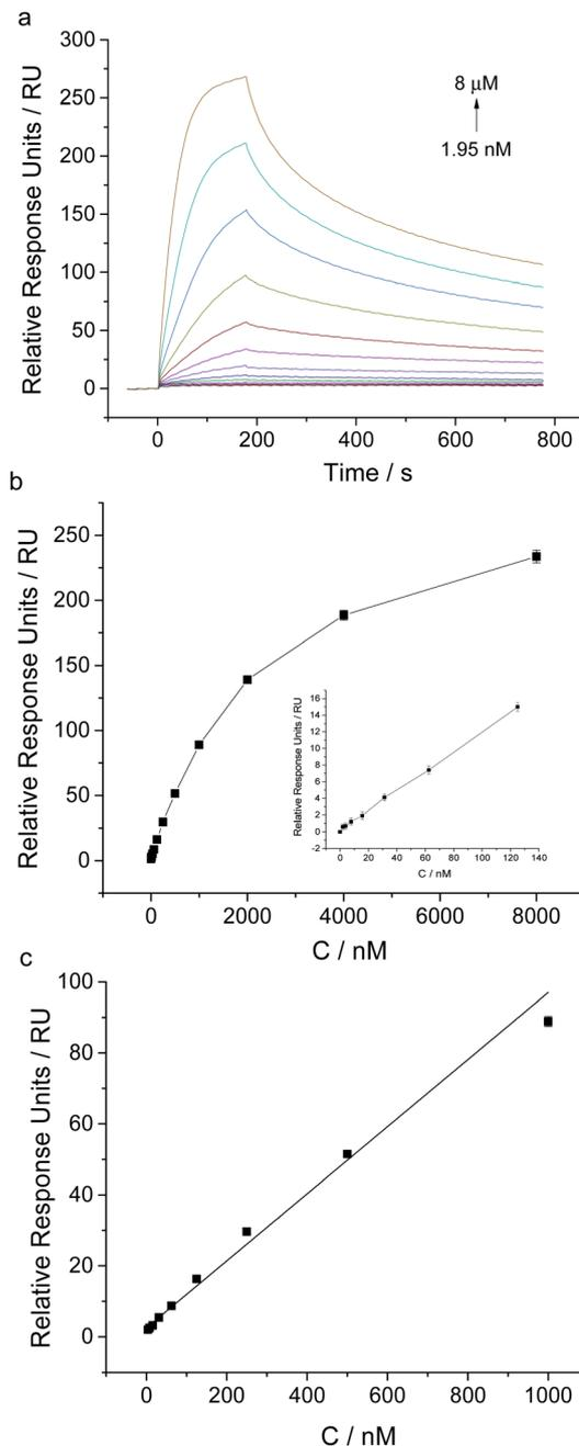
Fig. 4 SPR analysis of different concentrations of NSE using the aptamer coated chip. (a) Sensorgrams of the injection of NSE at different concentrations ranging from 1.95 nM to 8  $\mu\text{M}$ . (b) SPR response plot of the aptamer coated chip to different concentrations of NSE (inset: low concentrations ranging from 0 to 125 nM). (c) Calibration curve for NSE determination using this aptamer based SPR assay. Error bars are standard deviation for three independent determinations.
