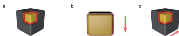
Fig. 9 Model A (a) and the structural diagram of the thermal conduction directions: parallel to the elongated Cu layer (b) and across the Cu layer (c).
