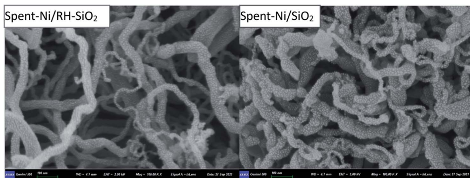
Fig. 10 SEM images of spent catalysts.
