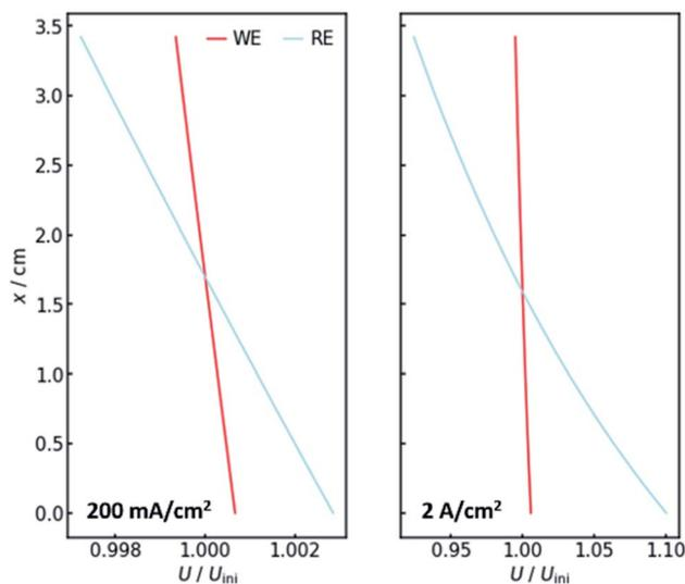
Fig. 5 The voltage drop at the working electrode (WE, red) and the potential as measured at the reference electrode position (RE, blue) for current densities of  $200 \text{ mA cm}^{-2}$  (left) and  $2 \text{ A cm}^{-2}$  (right) along the  $x$ -axis. All values are normalized by their value without gas evolution at the start of the iteration.
