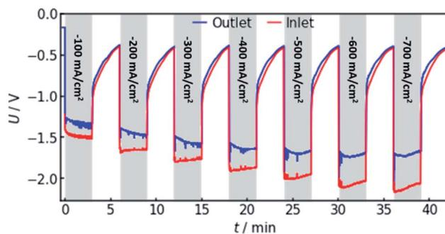
Fig. 6 Experimental measurement of the voltages at both the electrolyte inlet and outlet, using currents from  $-100$  to  $-700 \text{ mA cm}^{-2}$ . The red line represents the potential as measured by an Ag/AgCl reference electrode in the electrolyte inlet. A similar, simultaneous measurement at the electrolyte outlet is represented by the blue line. The voltage offset was determined as the difference of average measured potential at the two electrodes for each applied current density.
