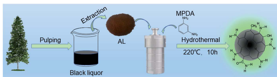
Scheme 1 Preparation process of NCQDs from alkaline lignin.
