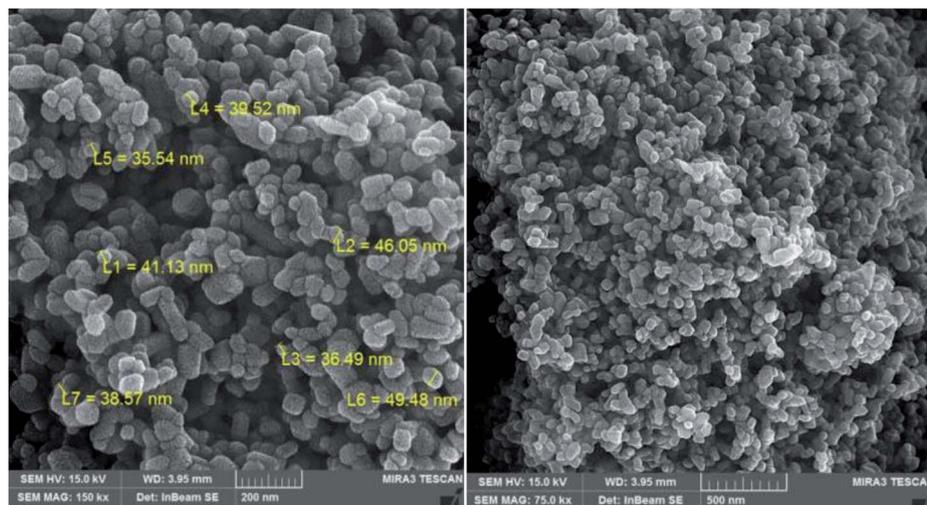
Fig. 8 SEM image of  $\gamma$ -Fe<sub>2</sub>O<sub>3</sub>@CPTMS-guanidine@SO<sub>3</sub>H.
