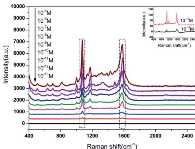
Fig. 5 SERS spectra of 4-ATP with different concentrations.
