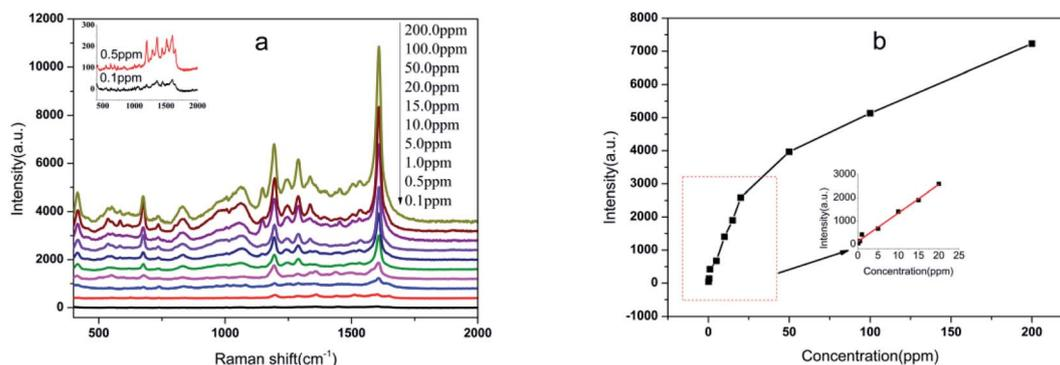
Fig. 7 (a) Typical SERS spectra of gradient concentrations of benzidine; (b) function of the peak intensity at  $1607\text{ cm}^{-1}$  of benzidine with concentration. Inset: a linear fitting for peak intensity at  $1607\text{ cm}^{-1}$  with the concentration ranging from 0.1 ppm to 20 ppm.
