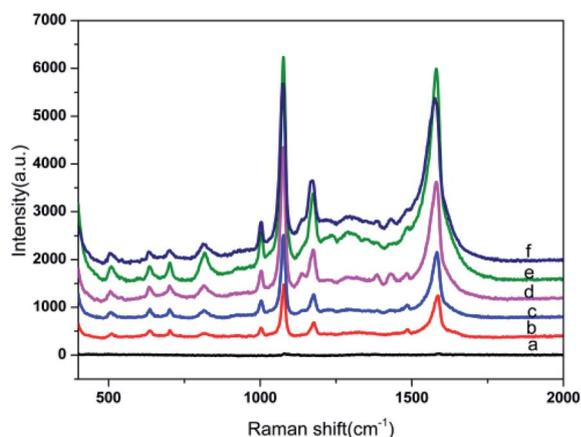
Fig. 4 SERS spectra of  $10^{-6}$  M 4-ATP using Au NPs-decorated filter paper substrate obtained at different electroless plating time: 0 min (a), 5 min (b), 10 min (c), 20 min (d), 40 min (e), and 60 min (f).
