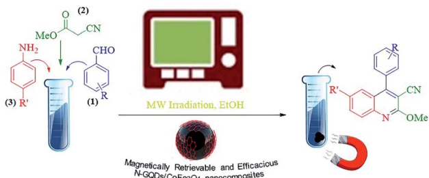
Scheme 1 MW-assisted synthesis of quinoline-3-carbonitrile frameworks.
