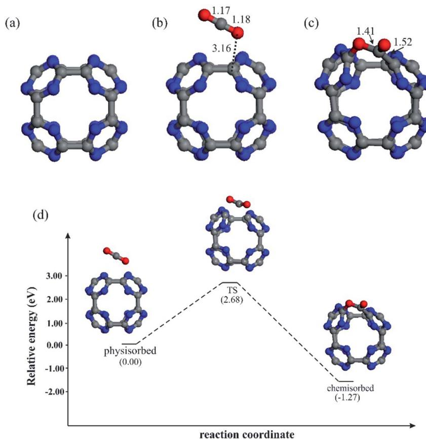
**Fig. 1** (a) The optimized structure of  $C_{24}N_{24}$ , (b) physisorbed structure of  $CO_2$  on  $C_{24}N_{24}$ , (c) chemisorbed structure of  $CO_2$  on  $C_{24}N_{24}$  and (d) the energy map for the physisorbed-to-chemisorbed transformation of  $CO_2$  on of  $C_{24}N_{24}$ . The color code of the atoms: O (red); C (gray); N (blue). The values on the optimized structures are bond distances (in Å).
