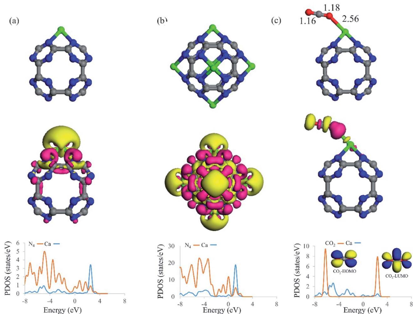
Fig. 2 The optimized structure (above), corresponding EDD (middle, isovalue = 0.002 au) and the PDOS plots of (a)  $\text{CaC}_{24}\text{N}_{24}$ , (b)  $\text{Ca}_6\text{C}_{24}\text{N}_{24}$  and (c)  $\text{CO}_2@ \text{CaC}_{24}\text{N}_{24}$ . In the EDD plots, the electron gain and loss regions are denoted by pink and yellow colors, respectively. The Fermi level in the PDOS plots is set to zero. The color code of the atoms: Ca (green); O (red); C (gray); N (blue).
