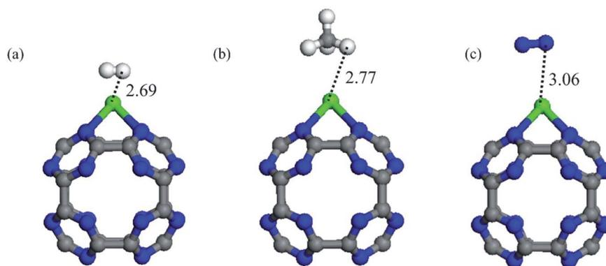
Fig. 5 The optimized structure and relevant bond distances (in Å) of the most stable configuration of (a) H<sub>2</sub>, (b) CH<sub>4</sub> and (c) N<sub>2</sub> adsorbed on CaC<sub>24</sub>N<sub>24</sub>.
