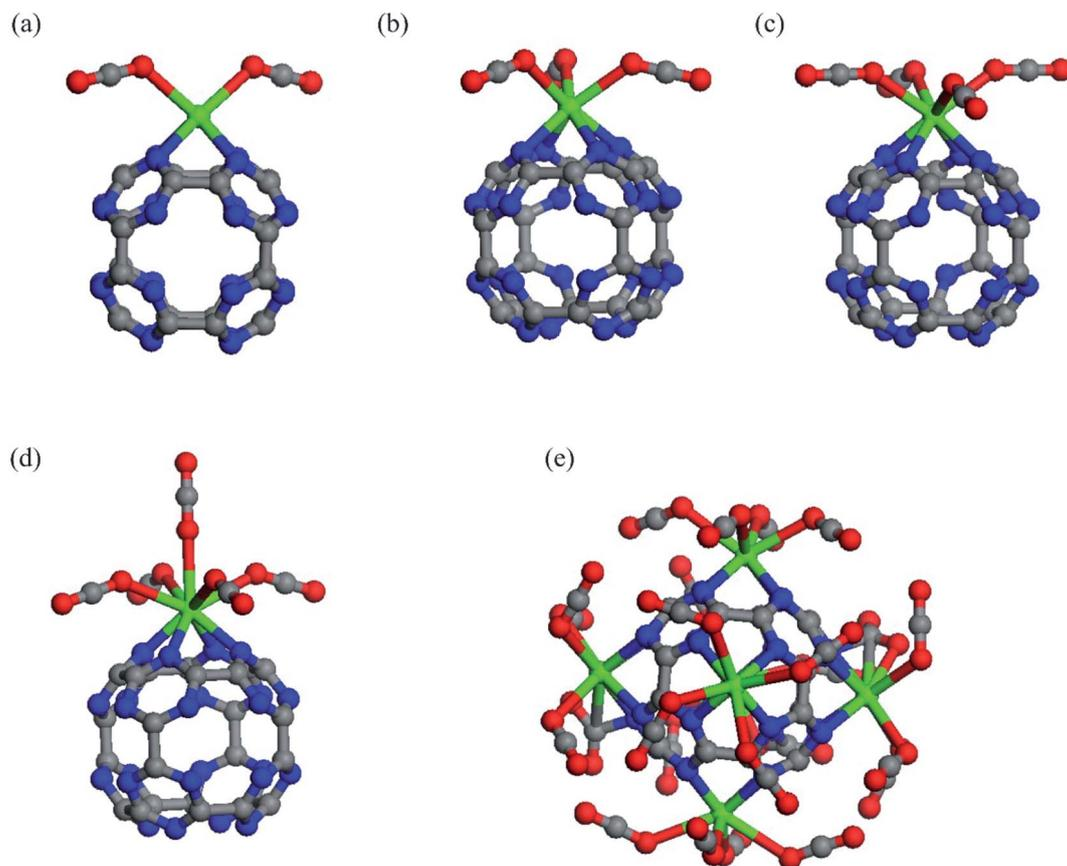
Fig. 4 The optimized structure of the most stable configuration of (a)  $2\text{CO}_2@CaC_{24}N_{24}$ , (b)  $3\text{CO}_2@CaC_{24}N_{24}$ , (c)  $4\text{CO}_2@CaC_{24}N_{24}$ , (d)  $5\text{CO}_2@CaC_{24}N_{24}$  and (e)  $24\text{CO}_2@Ca_6C_{24}N_{24}$  complexes. The color code of the atoms: Ca (green); O (red); C (gray); N (blue).
