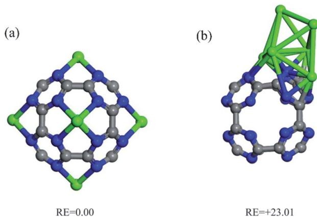
Fig. 3 Two stable isomers and correspond relative energy (RE, in eV) of Ca<sub>6</sub>C<sub>24</sub>N<sub>24</sub>: (a) Ca atoms are disperse on N<sub>4</sub> cavities of C<sub>24</sub>N<sub>24</sub> and (b) Ca atoms form a Ca<sub>6</sub> cluster on C<sub>24</sub>N<sub>24</sub>.
