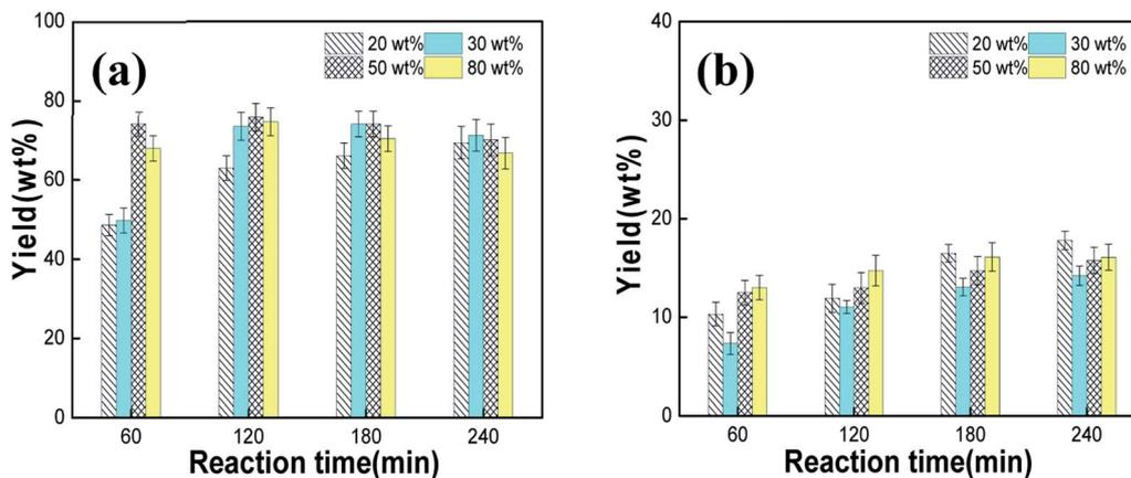
Fig. 5 Effect of the PMo<sub>12</sub> dosage on the starch degradation products: (a) monosaccharide yield; (b) glycolic acid yield.
