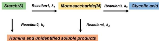
Scheme 1 Kinetic model of starch conversion over.
