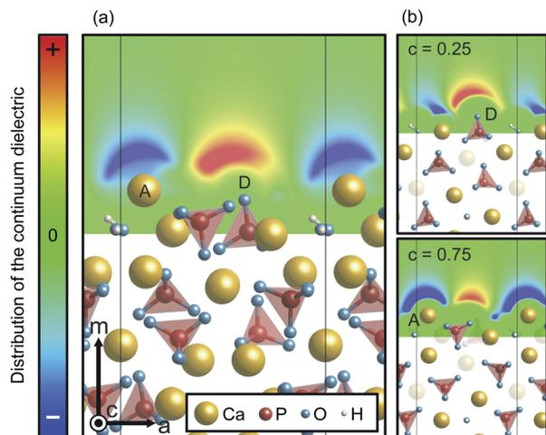
Fig. 6 Distribution of the continuum dielectric, which indicates the ionic charge density of the electrolyte, averaged along the  $c$  axis and (b) around O(D) and Ca(A) ions on the Ca-rich  $\{10\bar{1}0\}$  surface. For the color scheme, its maximum (colored red) and minimum (blue) values were set to  $1 \times 10^{-10}$  and  $-1 \times 10^{-10} \text{ e}^- \text{ \AA}^{-3}$ , respectively.
