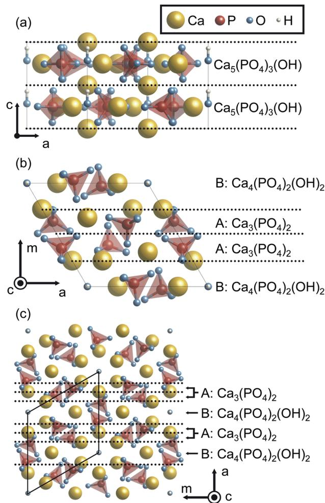
Fig. 1 HAp crystal structures viewed along the  $m$  and  $c$  axes. Stacking sequences of the atomic layers are indicated along the (a)  $c$ , (b)  $m$  and (c)  $a$  axes. The yellow, red, blue, and white balls represent Ca, P, O, and H atoms, respectively. In addition,  $\text{PO}_4$  groups are represented by tetrahedra. Each layer is separated by the dashed lines. The composition of each layer is also indicated.
