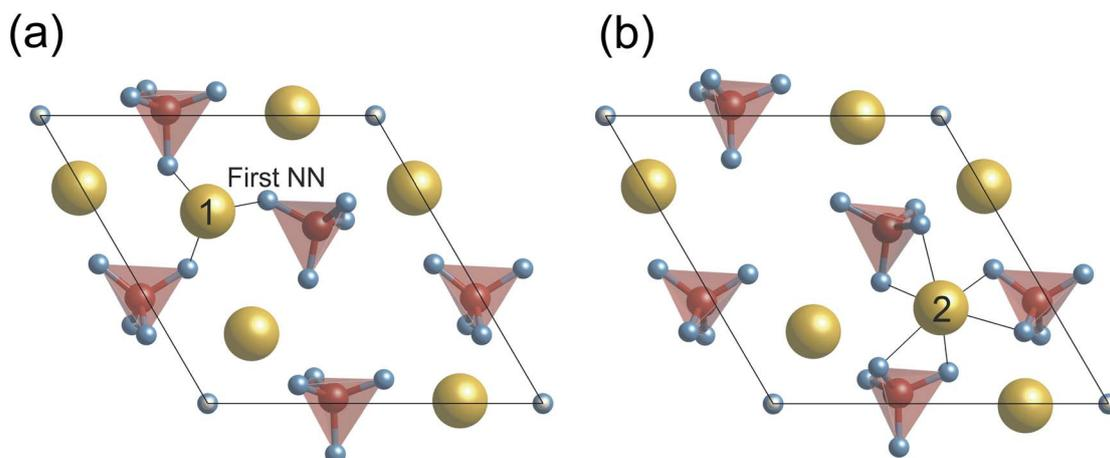
Fig. 4 Relaxed atomic configurations on the stoichiometric  $\{0001\}$  surfaces with  $\text{Ca}^{2+}$  at (a) site 1 and (b) site 2, which are relaxed under vacuum. For clarity, only ions on top of the  $\{0001\}$  surface are displayed.
