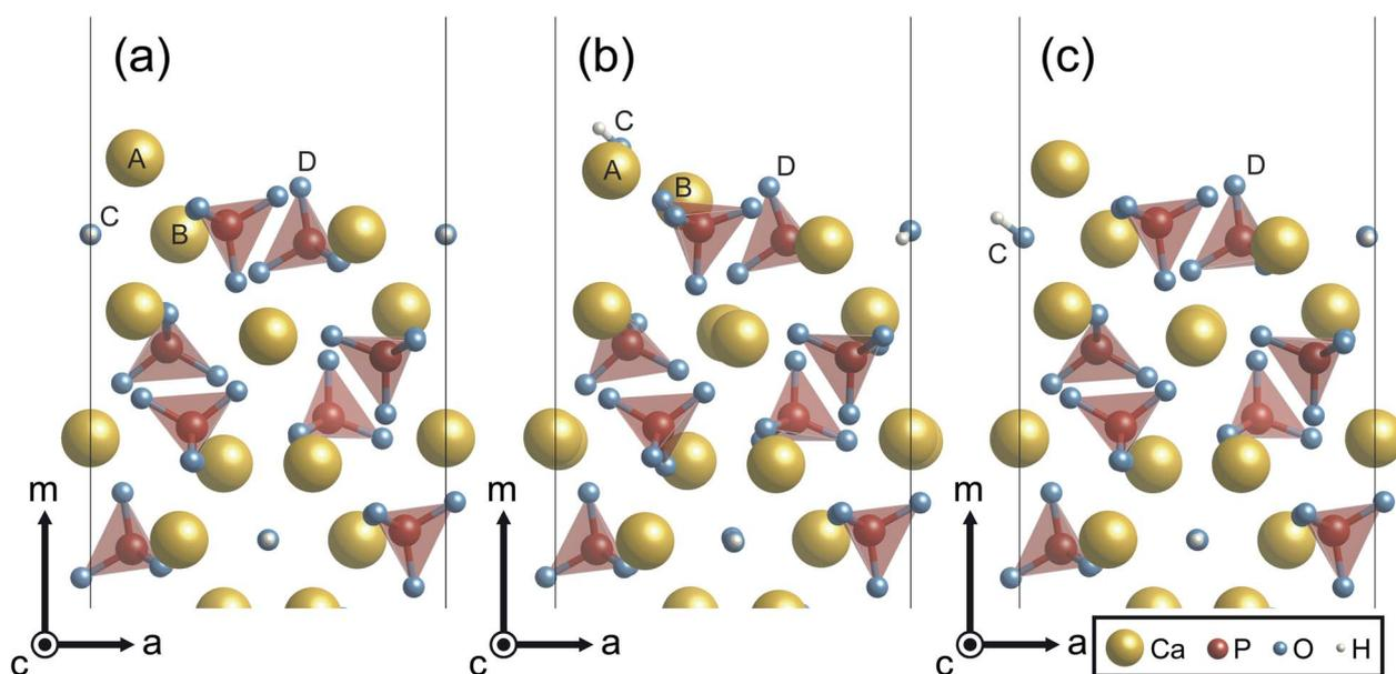
Fig. 5 Atomic configurations of the Ca-rich  $\{10\bar{1}0\}$  surface viewed along the  $c$  axis. (a) The unrelaxed structure, (b) the relaxed structure under vacuum, and (c) the relaxed structure with implicit solvation.
