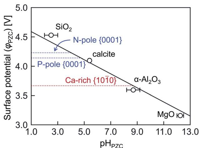
Fig. 8 Surface potentials  $\varphi_{\text{PZC}}$  plotted against  $\text{pH}_{\text{PZC}}$ . The solid line with a gradient  $-0.120$  V was obtained by least square regression according to the theoretical linear function proposed in ref. 45.
