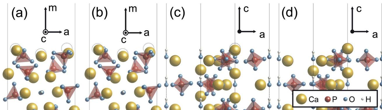
Fig. 7 Relaxed atomic structures of P-rich  $\{10\bar{1}0\}$  and P-pole  $\{0001\}$  surfaces. (a) Relaxed P-rich  $\{10\bar{1}0\}$  under vacuum, (b) relaxed P-rich  $\{10\bar{1}0\}$  in the implicit solvation, (c) relaxed P-pole  $\{0001\}$  under vacuum, (d) relaxed P-pole  $\{0001\}$  in the implicit solvation. Broken circles indicate original Ca positions before relaxation.
