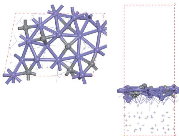
Fig. 1 Top (left) and side (right) views of hcp-Fe<sub>7</sub>C<sub>3</sub> (211) surface (blue: Fe atoms; gray: C atoms).
