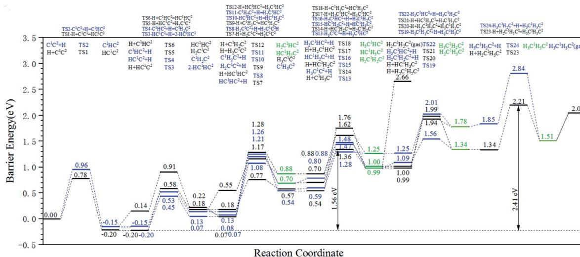
Fig. 4 Energy profile diagram for the stepwise hydrogenation pathway of  $C_2$  species on the hcp- $Fe_7C_3$  (211) surface. Black lines: hydrogenation reactions occurring on  $C^1$ . Blue lines: hydrogenation reactions occurring on  $C^2$ . Green lines: products from both kinds of hydrogenation reactions.
