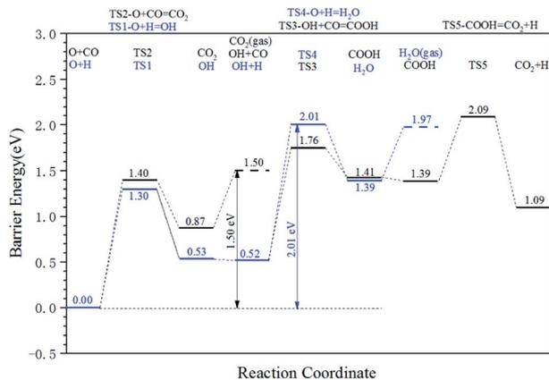
Fig. 6 Energy profile diagram for oxygen removal pathways on hcp-Fe<sub>7</sub>C<sub>3</sub> (211). Blue lines: the H<sub>2</sub>O formation pathways. Black lines: the CO<sub>2</sub> formation pathways.
