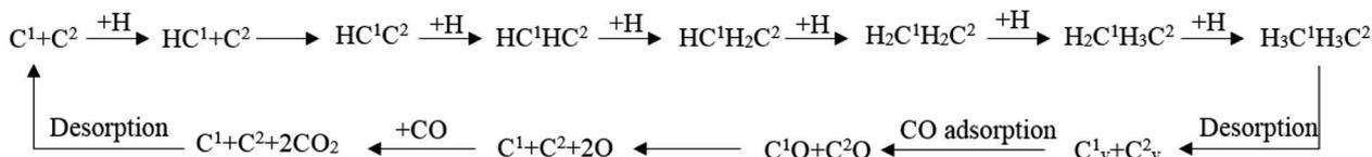
Scheme 6 The full map of the Fischer–Tropsch mechanism on hcp-Fe<sub>7</sub>C<sub>3</sub> (211).
