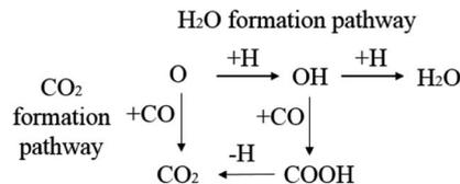
**Scheme 5** The designed oxygen removal pathways on hcp-Fe<sub>7</sub>C<sub>3</sub> (211).
