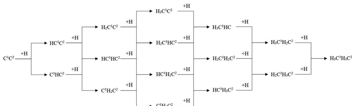
Scheme 3 The designed stepwise hydrogenation pathway of C<sub>2</sub> species on hcp-Fe<sub>7</sub>C<sub>3</sub> (211).
