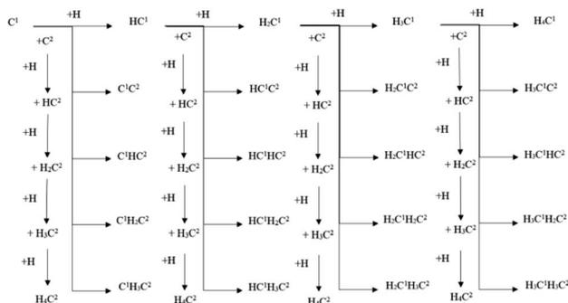
**Scheme 1** The designed C<sup>1</sup>-C<sup>2</sup> coupling pathways on hcp-Fe<sub>7</sub>C<sub>3</sub> (211).
