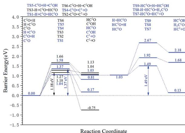
**Fig. 5** Energy profile diagram for the carbon vacancy recovery pathway on defect-hcp-Fe<sub>7</sub>C<sub>3</sub> (211). Blue lines: the carbon vacancy recovery pathway in the Cv1 site. Black lines: the carbon vacancy recovery pathway in the Cv2 site.
