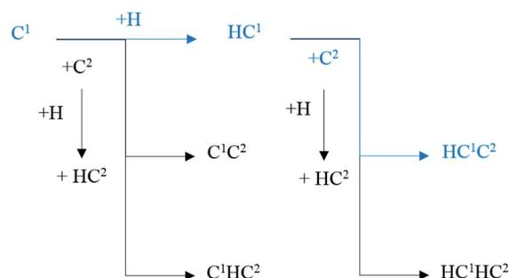
Scheme 2 The major  $C^1$ - $C^2$  coupling pathways (black lines) and preferred  $C^1$ - $C^2$  coupling pathways (blue lines) on hcp-Fe<sub>7</sub>C<sub>3</sub> (211).
