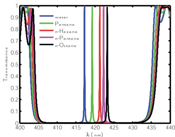
**Fig. 3** Transmittance of the proposed design [air/(SiO<sub>2</sub>/ZnO)<sup>N</sup>/cavity/(SiO<sub>2</sub>/ZnO)<sup>N</sup>/glass] with different organic samples at normal incidence. The thickness of the cavity is 840 nm.
