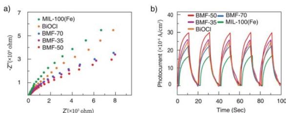
Fig. 6 (a) Nyquist impedance plots and (b) transient photocurrent responses of the samples.
