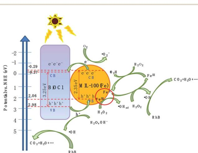
Fig. 9 Photo-Fenton catalytic mechanism of BiOCl/MIL-100(Fe) under visible-light illumination.
