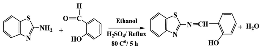
Scheme 1 The preparation of the Schiff base BTMP (ionophore).
