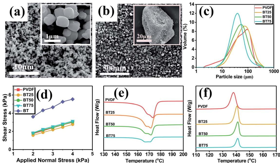
Fig. 2 SEM images of (a) BaTiO<sub>3</sub> and (b) BT50 powder. (c) The particle size distribution curves of PVDF and PVDF/BaTiO<sub>3</sub> powder. (d) The shear test curves of PVDF, BaTiO<sub>3</sub> and PVDF/BaTiO<sub>3</sub> powder. The DSC thermograms of the powder: (e) the heating process and (f) the cooling process.
