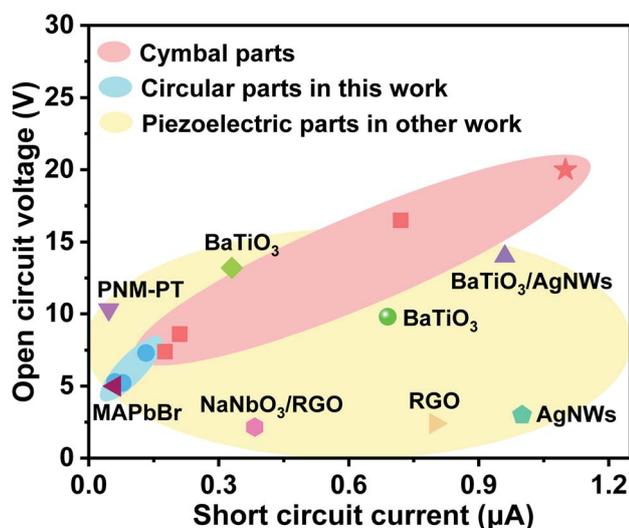
Fig. 6 The comparison of the piezoelectric performance between cymbal structure parts, circular parts and other reported PVDF-based composite parts (the respective composited piezoelectric ceramics are indicated).
