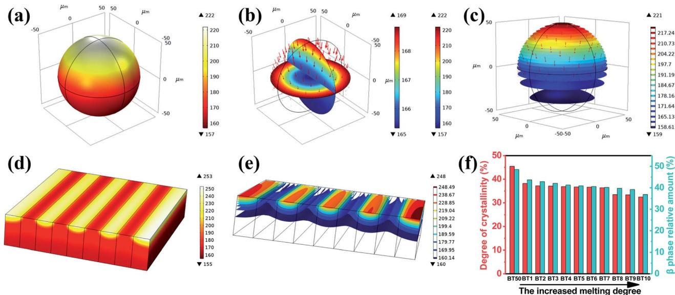
Fig. 4 The finite element analysis of the powder's heat conduction behavior under laser irradiation: (a) surface, (b) section and (c) isothermal surface. The finite element analysis of the powder bed's heat conduction behavior under laser irradiation: (d) surface and (e) isothermal surface. (f) The crystallinity and  $\beta$  phase relative amount of the PVDF/BaTiO<sub>3</sub> composites with different melting degrees.
