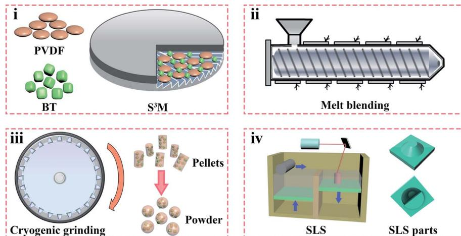
Fig. 1 A schematic illustration of the process for the preparation and SLS processing of the PVDF/BaTiO<sub>3</sub> composites.
