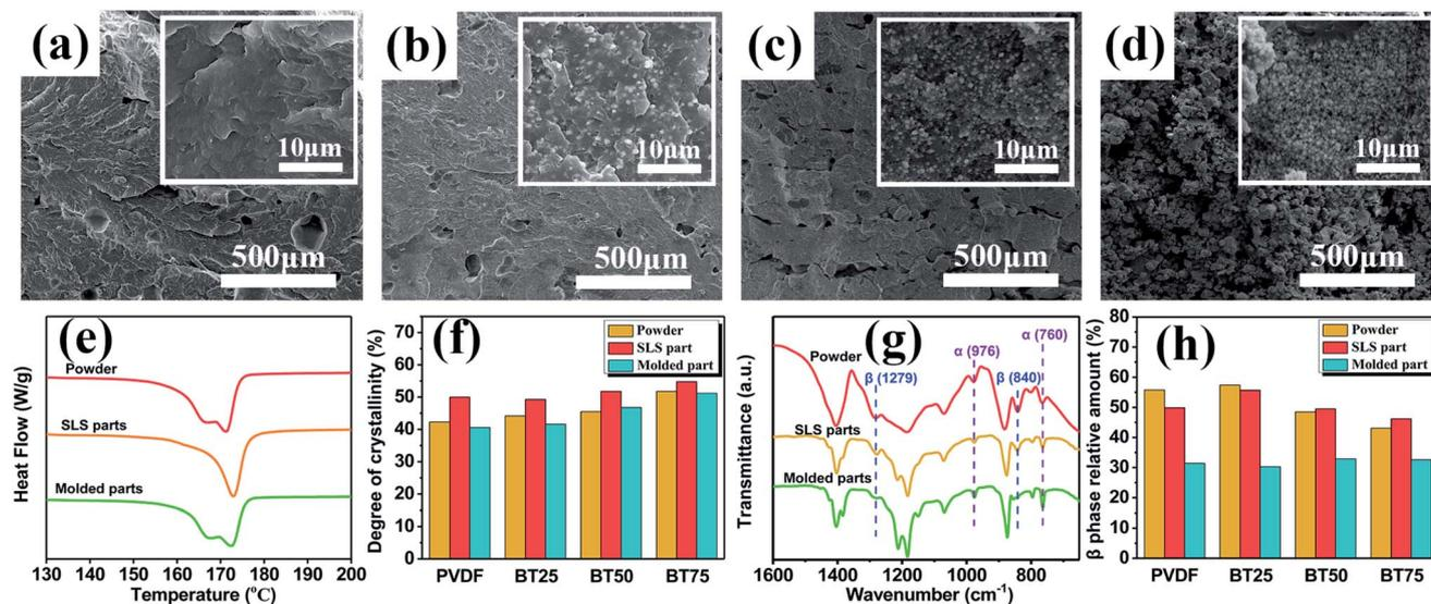
Fig. 3 The SEM images of fractured surfaces of the SLS parts: (a) PVDF, (b) BT25, (c) BT50 and (d) BT75. (e) The DSC curves of the powder, SLS parts and molded parts at the BaTiO<sub>3</sub> content of 50 wt%, and (f) the crystallinity of the powder, SLS parts and molded parts. (g) The FT-IR spectra of the powder, SLS parts and molded parts at the BaTiO<sub>3</sub> content of 50 wt%, and (h) the  $\beta$  phase relative amount of the powder, SLS parts and molded parts.
