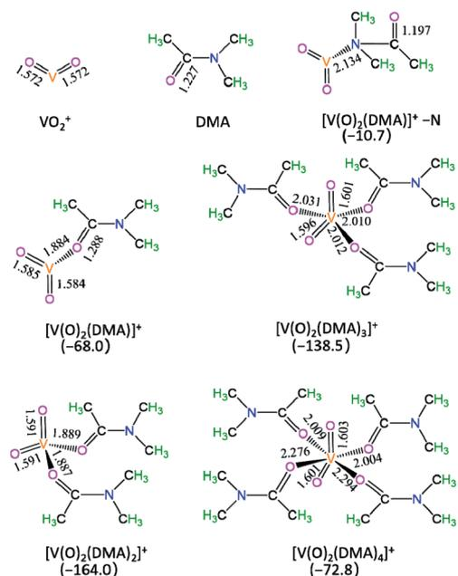
Fig. 1 The optimized geometric structures and the formed Gibbs free energies ( $G_r$ ,  $\text{kJ mol}^{-1}$ ) of  $[\text{V}(\text{O})_2(\text{DMA})_x]^+$  complexes in the DMA solution. Bond lengths are reported in Å.
