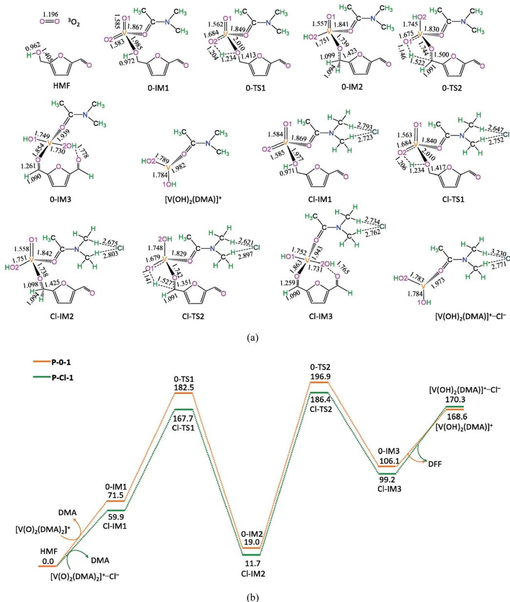
Fig. 2 The geometric structures (a) and the schematic energy diagrams (b) with the relative Gibbs free energy ( $G_r$ , kJ mol<sup>-1</sup>) relative to the reactants for the first HMF oxidation to DFF catalyzed by  $[\text{V}(\text{O})_2(\text{DMA})_2]^+$  without/with  $\text{Cl}^-$  in the DMA solution. For clarity, the hydrogen atoms on carbon are not shown. Bond lengths are reported in Å.
