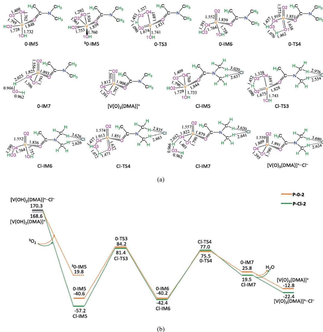
Fig. 3 The geometric structures (a) and the schematic energy diagrams (b) with the relative Gibbs free energy ( $G_r$ , kJ mol<sup>-1</sup>) relative to the reactants for the oxidative dehydration of  $[V(OH)_2(DMA)]^+$  to  $[V(O)_3(DMA)]^+$  catalyzed by without/with  $Cl^-$  in the DMA solution. For clarity, the hydrogen atoms on carbon are not shown. Bond lengths are reported in Å.
