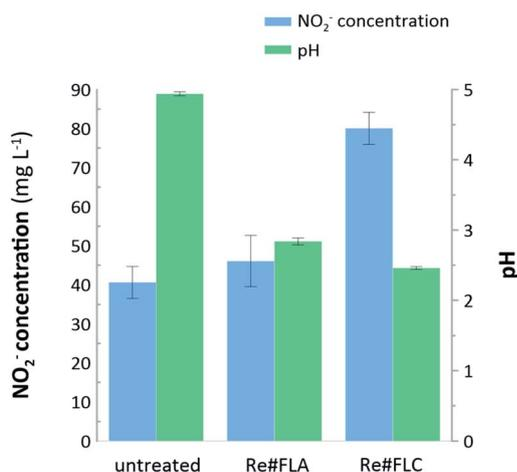
Fig. 4 Concentration of NO<sub>2</sub><sup>-</sup> ions and the pH determined in the untreated, FLC-dc-APGD-treated, and FLA-dc-APGD-treated Re-based nanostructures precursor solutions.
