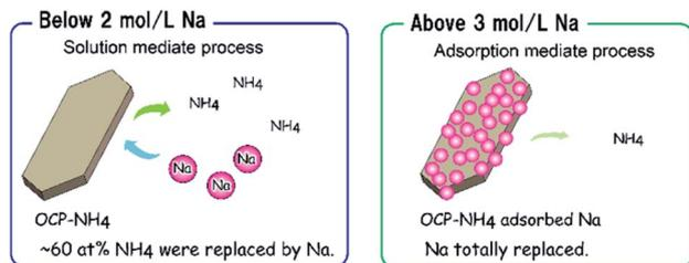
Scheme 2 Schematic of the ion-exchange process of OCP-NH<sub>4</sub> in systems with different Na concentrations.
