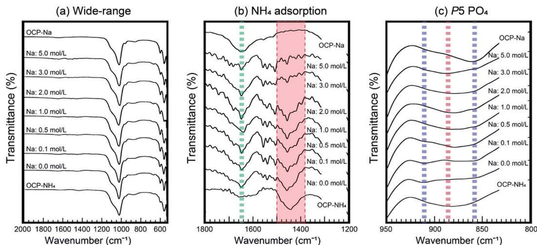
Fig. 7 FT-IR spectra of the treated samples: (a) wide-range spectra; (b) region of  $\text{NH}_4$  adsorption bands, showing the  $\text{HPO}_4$  band (green broken line) and the  $\text{NH}_4$  adsorption band (red shaded region); (c) region of  $P5\text{ PO}_4$ , showing the bands corresponding to cation adsorption of OCP- $\text{NH}_4$  (red broken line) and OCP-Na (blue broken lines).
