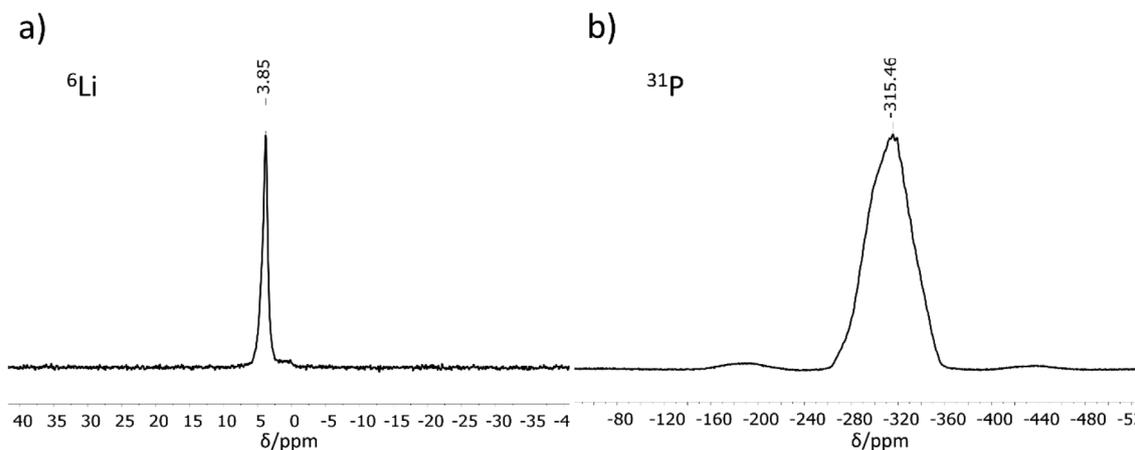
**Fig. 2**  $^6\text{Li}$  (a) and  $^{31}\text{P}$  (b) MAS-NMR measurements performed for  $\text{Li}_3\text{InP}_2$ .
