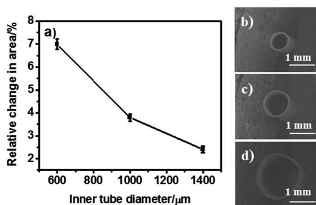
Fig. 3 (a) Relative maximum cross-sectional area change as a function of the inner tube diameter in 0.5 M  $\text{LiClO}_4$ . SEM images of tubes with different inner diameters (b) 600  $\mu\text{m}$  (c) 1000  $\mu\text{m}$  and (d) 1400  $\mu\text{m}$ .
