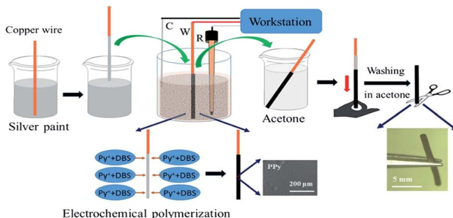
**Scheme 1** Synthesis of tubular polypyrrole actuators. C: counter electrode, R: reference electrode and W: working electrode for electrochemical polymerization of pyrrole (Py) to synthesize polypyrrole (PPy) doped with dodecyl benzenesulfonate (DBS) anions. The electron microscopy picture shows the surface of the generated PPy tube. The optical image illustrates the final polymer tube after removal of the template wire.
