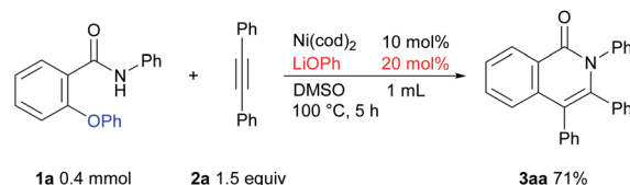
Scheme 7 The reaction using a catalytic amount of \text{LiOPh} .
