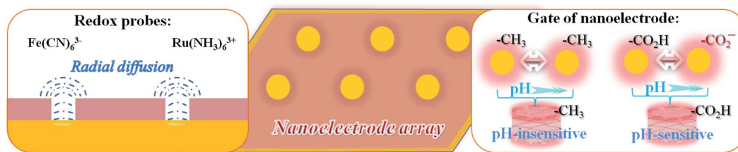
Scheme 1 Illustrations of radial diffusion at the nanoelectrode arrays, and pH-sensitive and insensitive interfacial characteristics.
