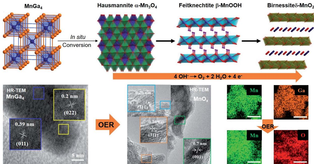
Fig. 10 Proposed mechanism for the electroconversion of MnGa<sub>4</sub> to δ-MnO<sub>2</sub> with its intermediates (top). TEM images of MnGa<sub>4</sub> and the transformed oxide species after OER in alkaline media (bottom left). EDX mapping of Mn and Ga in MnGa<sub>4</sub> before alkaline OER and Mn and O mapping after. Adapted with permission from ref. 97, copyright 2019, Wiley-VCH.
