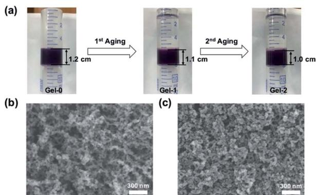
Fig. 2 (a) Pictures of the gel shrinkage during first two aging cycles. SEM images of (b) **Aerogel-0** and (c) **Aerogel-2**.
