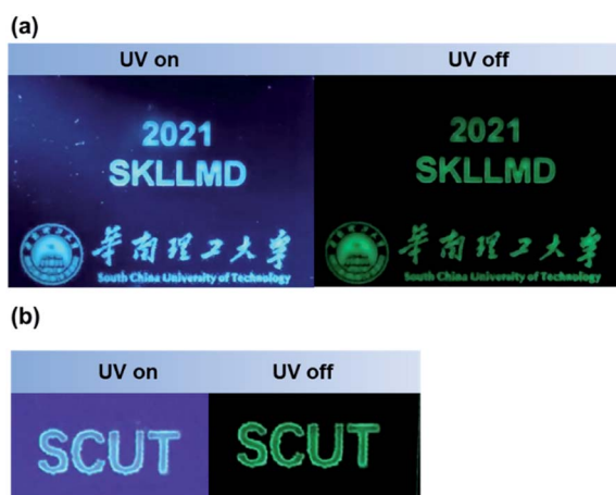
Fig. 3 A demonstration of confidential encryption: photographs of BTPO-BCN in PMMA film (a) in an inert gas and (b) covered by PVA in air under a UV lamp (left) and after the removal of the UV source (right).
