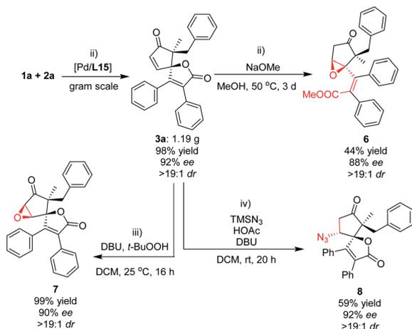
Fig. 6 Synthetic application of the oxaspiro cyclopentenone–lactone scaffold for the downstream transformations. (i) Gram-scale synthesis of **3a**; (ii) transesterification-induced intramolecular oxa-Michael addition; (iii) epoxidation reaction for the enantioselective synthesis of **7** bearing an additional epoxide; (iv) conjugate addition reaction of TMSN<sub>3</sub>/HOAc for the enantioselective synthesis of **8** bearing an additional azide.
