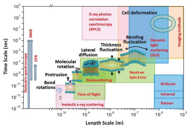
Fig. 1 Schematic diagram of lipid membrane dynamics accessible by neutron spectroscopic techniques over different length and time scales (reproduced with permission from Qian *et al.*, *Langmuir*, **36**, 15189–15211.<sup>63</sup> Copyright 2020 American Chemical Society).
