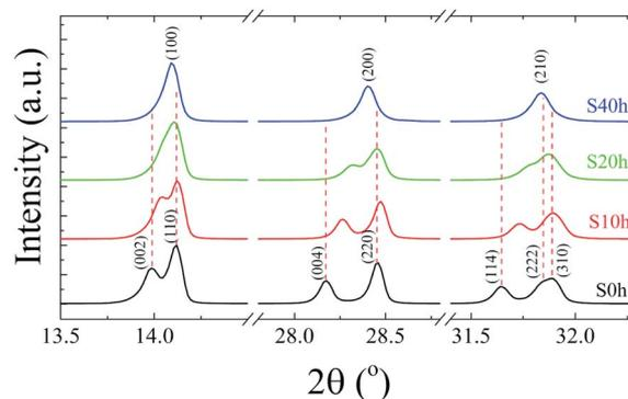
Fig. 2 Room-temperature X-ray diffraction patterns of the pelletized  $\text{MAPbI}_3$  sample after being submitted to a heat treatment at  $T = 250 \text{ }^\circ\text{C}$  for different annealing times,  $t = 0, 10, 20,$  and  $40 \text{ h}$ .
