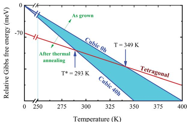
Fig. 8 Schematic of the Gibbs free energy as a function of temperature. At  $T = 0$  K, the energies correspond to the internal energy of each system and were computed within the DFT approach and used the cubic system as a reference. As the temperature increases, the configuration entropy is responsible for different phase transition temperatures from tetragonal to cubic, indicated by 293 and 349 K. The configurational entropy is larger for the sample that was annealed for 40 h.
