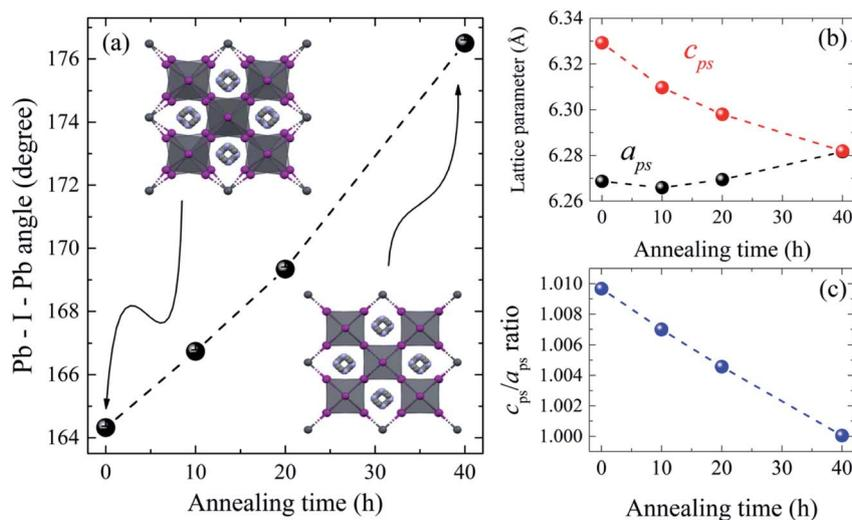
**Fig. 5** Structural parameters of the MAPbI<sub>3</sub> samples submitted to thermal annealing at 250 °C (523 K) and different annealing time. (a) The Pb–I–Pb bond angle changing to almost 180°; insets illustrate rotation of PbI<sub>6</sub> octahedra along the  $c$ -axis. (b) Pseudocubic lattice parameters and (c) variation of lattice parameter ratio,  $c_{\text{ps}}/a_{\text{ps}}$ , which reaches 1 for 40 h annealing time.
