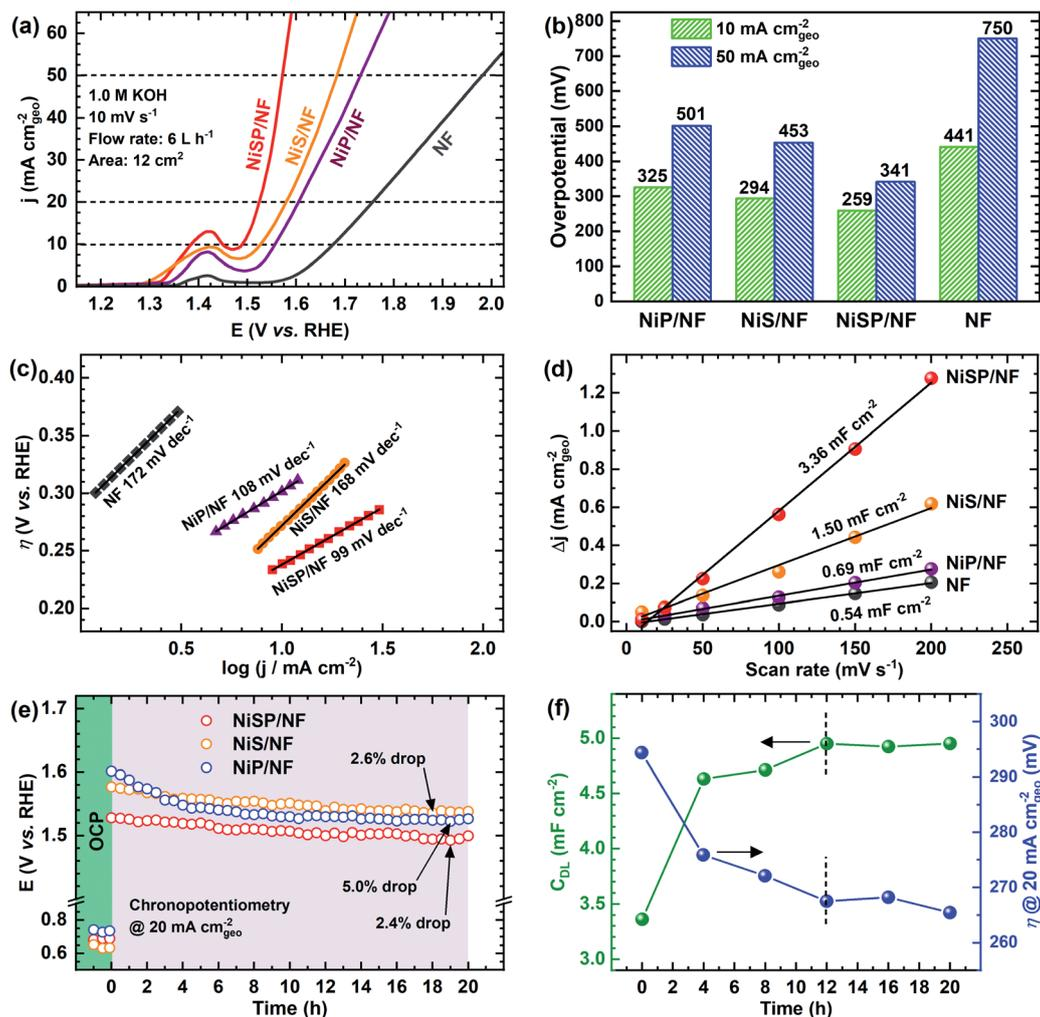
Fig. 4 OER electrochemical characterization results: (a) anodic  $i$ - $V$  curves, (b) overpotentials at 10 and 50 mA cm<sup>-2</sup>, (c) Tafel slopes, (d) double-layer capacitances and (e) chronopotentiometric runs at 20 mA cm<sup>-2</sup> during a period of 20 h, using the as-prepared electrodes in 1 M KOH electrolyte. (f) Double layer capacitance and overpotential at 20 mA cm<sup>-2</sup> of the NiSP/NF electrode with time.
