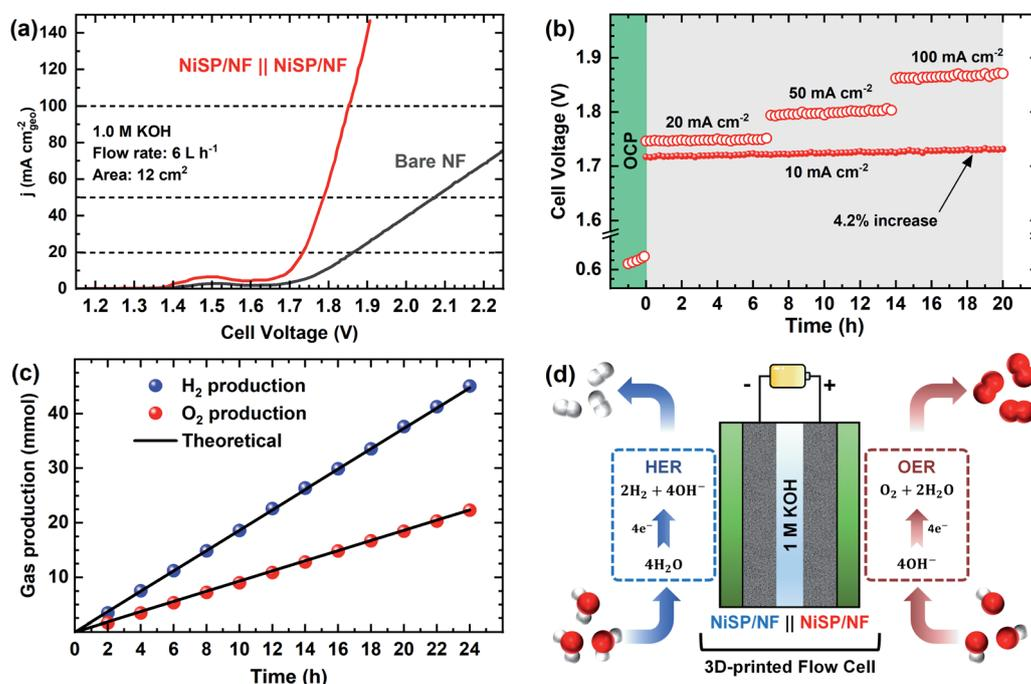
Fig. 8 Overall water splitting results: (a) *i*-V curves, (b) chronopotentiometric run at different current densities for 20 h, (c) gas evolution measurements at  $10 \text{ mA cm}^{-2}$ , and (d) schematic illustration of the assembled flow cell with NiSP/NF electrodes using 1 M KOH electrolyte.
