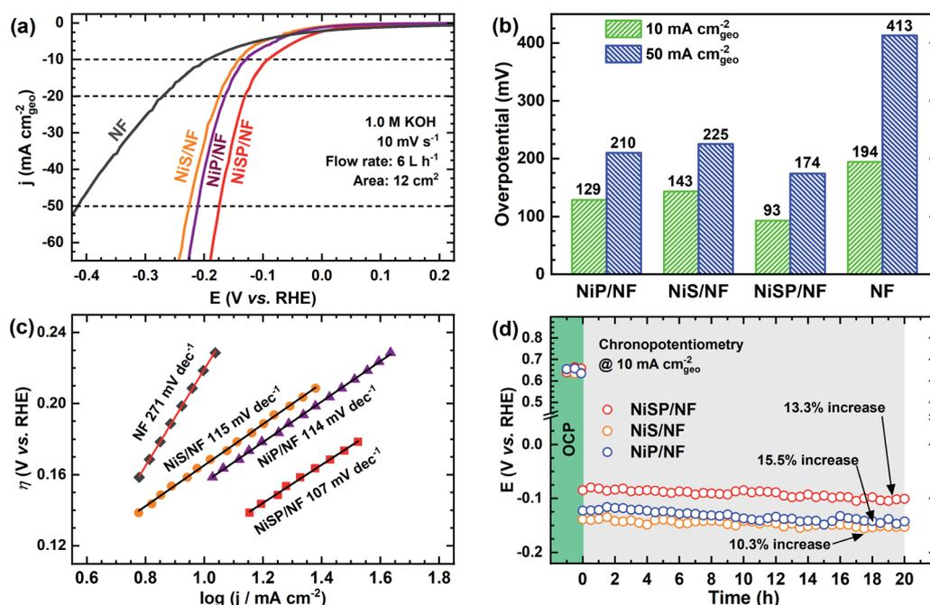
Fig. 5 HER electrochemical characterization results: (a) cathodic  $i$ - $V$  curves, (b) overpotentials at 10 and 50 mA cm<sup>-2</sup>, (c) Tafel slopes, and (d) chronopotentiometric runs at 10 mA cm<sup>-2</sup> for 20 h using the as-prepared electrodes in 1 M KOH electrolyte.
