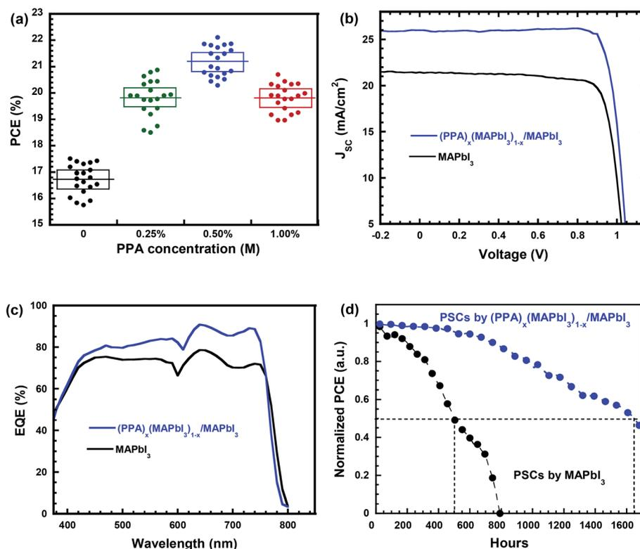
Fig. 3 (a) The statistics of the PCE of the PSCs with  $(\text{PPA})_x(\text{MAPbI}_3)_{1-x}/\text{MAPbI}_3$  thin films with different PPA concentrations. (b) The  $J$ - $V$  characteristics and (c) EQE spectra of PSCs with either the  $\text{MAPbI}_3$  or  $(\text{PPA})_x(\text{MAPbI}_3)_{1-x}/\text{MAPbI}_3$  thin films. (d) The stabilities of the PSCs with either the  $\text{MAPbI}_3$  thin film or the  $(\text{PPA})_x(\text{MAPbI}_3)_{1-x}/\text{MAPbI}_3$  thin film.
