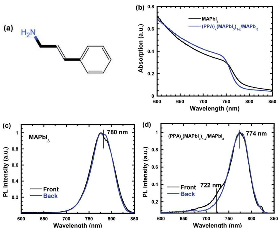
Fig. 1 (a) The molecular structure of PPA. (b) The absorption spectra of the  $\text{MAPbI}_3$  and  $(\text{PPA})_x(\text{MAPbI}_3)_{1-x}/\text{MAPbI}_3$  thin films. The PL spectra of the (c)  $\text{MAPbI}_3$  and (d)  $(\text{PPA})_x(\text{MAPbI}_3)_{1-x}/\text{MAPbI}_3$  thin films from the front side and back side.
