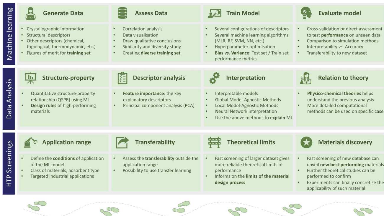
Fig. 3 Schematic representation of the main subjects typically covered as part of an ML-assisted high-throughput screening procedures. First, one needs to train a machine learning (ML) model and analyse its performance on an independent subset of the data. Then, one can use the model to quantitatively extract structure–property relationships. Finally, once proven accurate, the model can be used on a larger scale to accelerate screening procedures.
