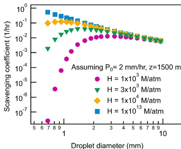
Fig. 3 Scavenging coefficient as a function of droplet size for monodisperse droplets assuming a constant precipitation intensity and height ( $P_0 = 2$  mm h<sup>-1</sup> and  $z = 1500$  m). Each color represents a different Henry's law constant ( $H$ ).
